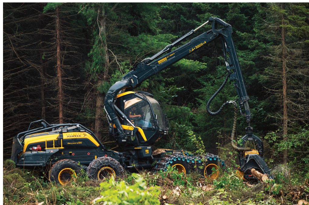
Pine pulp is harvested and cut to length with a Ponsse Scorpion King harvester.
