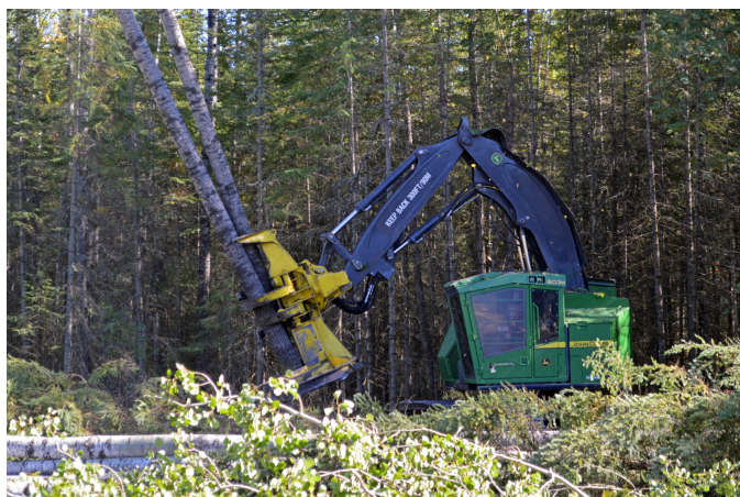
Kirk Lindberg harvests aspen with a John Deere 803M feller buncher. L&L also utilizes a Komatsu XT430.
