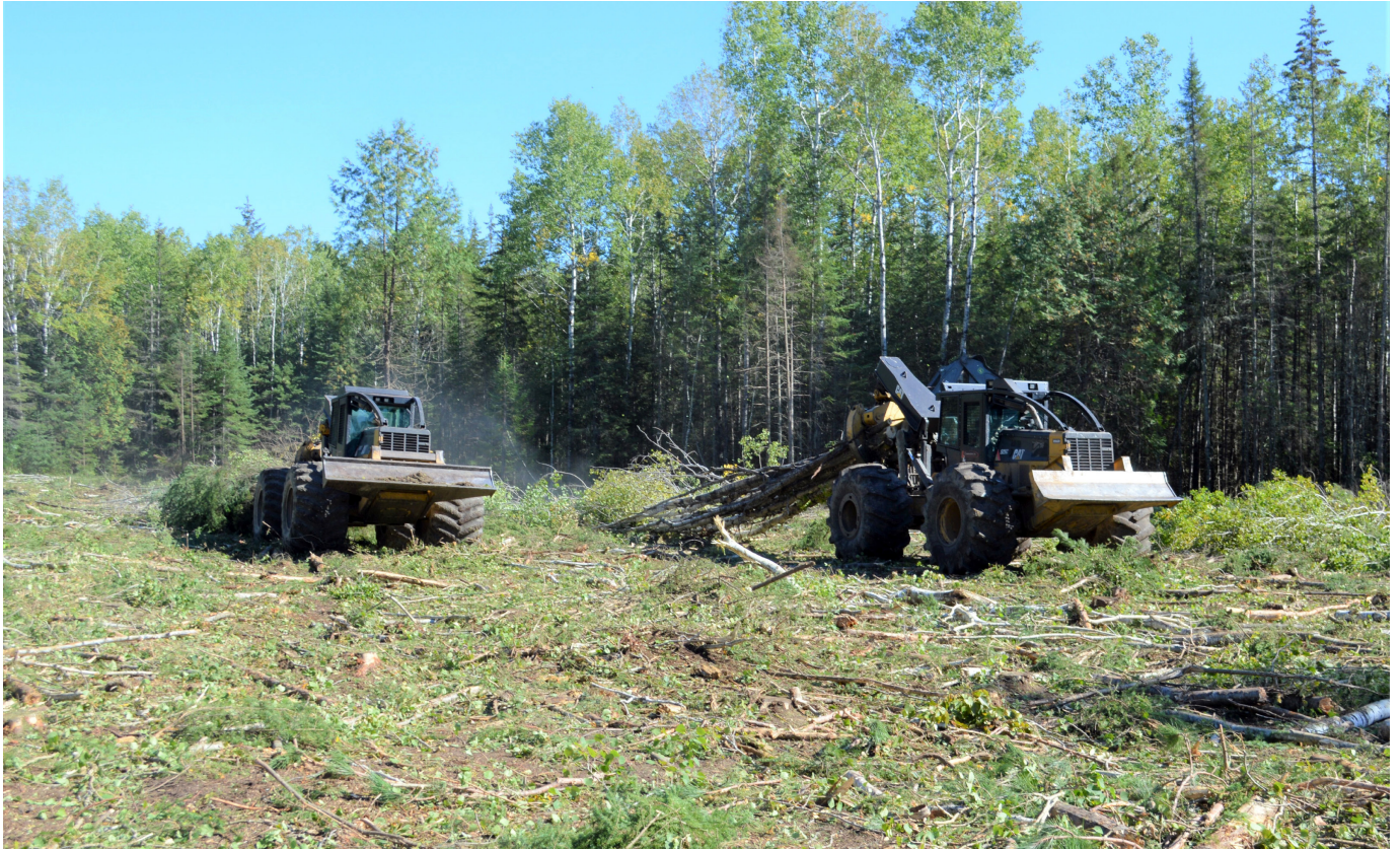
Two Cat 525C skidders—driven by Jason Nygaard and Nate Lynch—drag harvested timber to the landing for processing.
