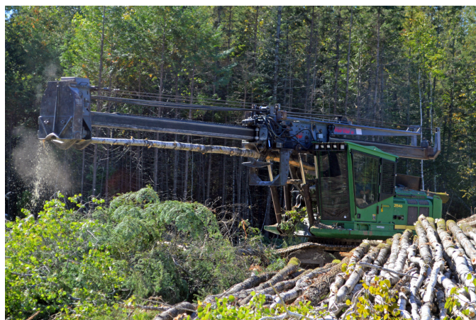
Blake McBride operates a John Deere 2154D stroke delimeter with a 453 ProPac boom.
