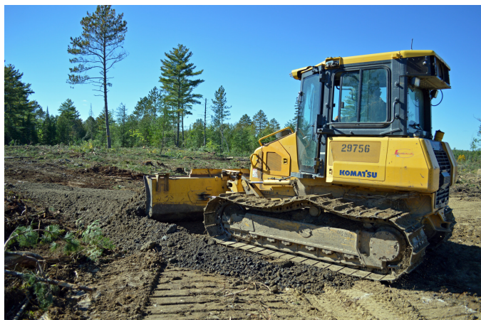
Nick Lagen builds roads and landings with a Komatsu dozer. L&L also has a Cat D5k2 dozer.
