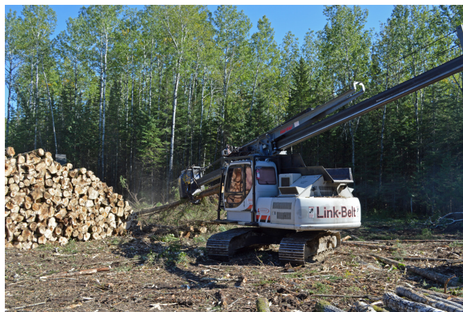
This Link-Belt 210LX delimeter with a 453 ProPac boom operated by Lloyd Stavish. L&L has a total of three delimeters—2 Link-Belts and a John Deere—two of which are utilized on most sites.
