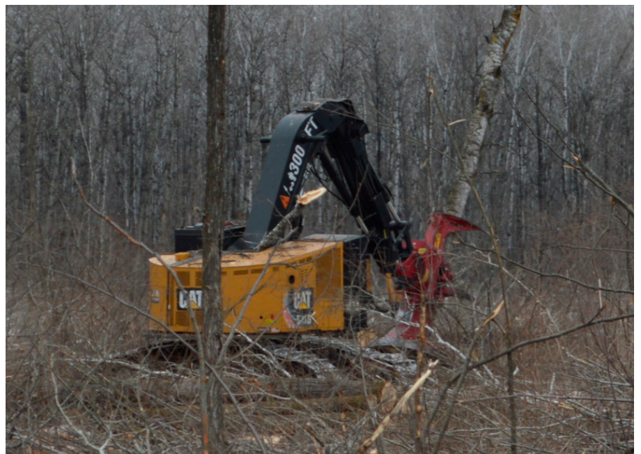
Cory Aho harvests aspen with a CAT 521B feller buncher for J&A Logging.
