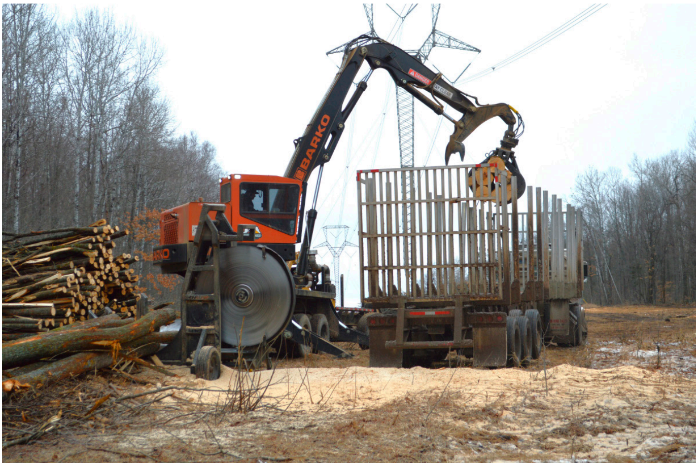
Jesse Anderson utilizes a Barko 495B to load a truck for delivery to the mill.
