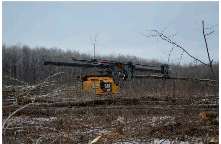
Mike Johnson maneuvers a CAT 538 throughout the harvest site to delimit harvested timber for J&A Logging.
