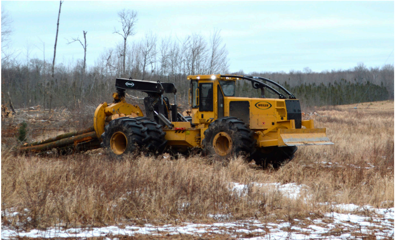
Jacob Anderson drives a Weiler S550 skidder, equipped with dual tires on the rear to minimize its impact on soil conditions.
