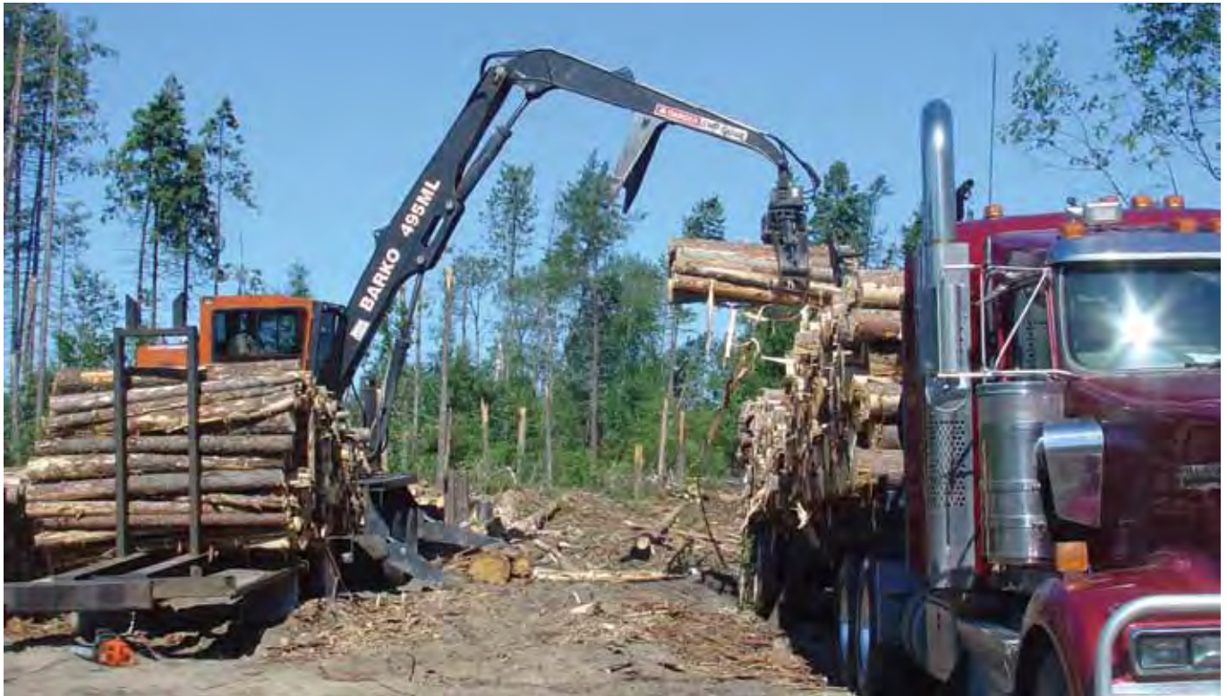
Rod Gerbracht loads timber after slashing it with a Barko 495. He likes to run the slasher/loader so he can stay on the landing and manage the trucks that come and go on the logging job.
