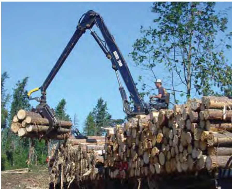
Mitch Johannessohn uses a center-mount to load timber for delivery to the mill.
