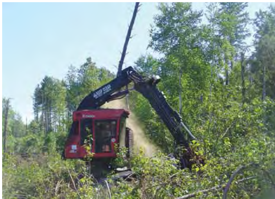
Sawdust flies as Dave Gerbracht operates the Timbco feller buncher in blown down timber.
