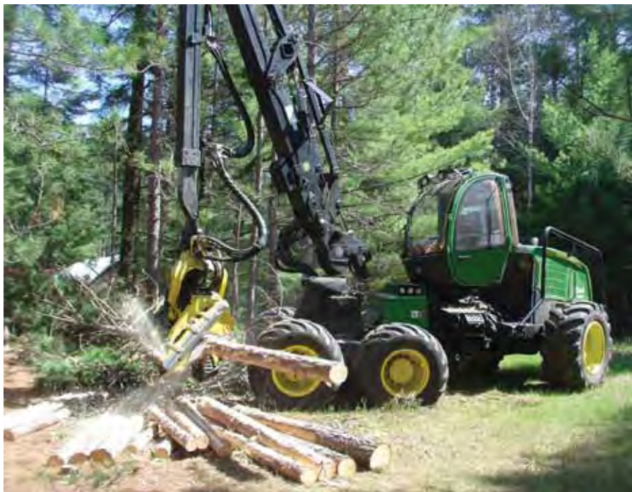
Scott Pittack thins red pine with a John Deere 1270E harvester.
