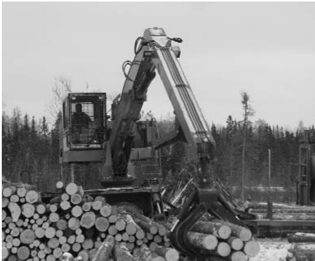
Kainz operates his slasher at a jobsite just west of Babbitt. He uses a 200 Serco loader on an International truck with a slasher unit.
