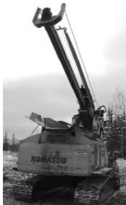
Kainz uses a Komatsu delimeter. He also utilizes a Dimarco for delimiting. His bunchers usually work as much as a week ahead of the rest of his equipment.
