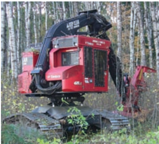
Corey Lovdahl runs the company's Timbco 425 EXL buncher. This sale is predominantly aspen, with some balsam spruce and a little birch.
