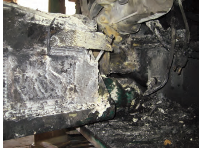
The batteries, electrical wiring, and starter area were damaged on this feller buncher.
