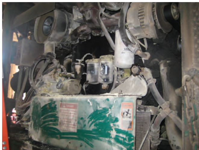
The main fire was located behind the battery cover, involving the batteries and surrounding engine area.
