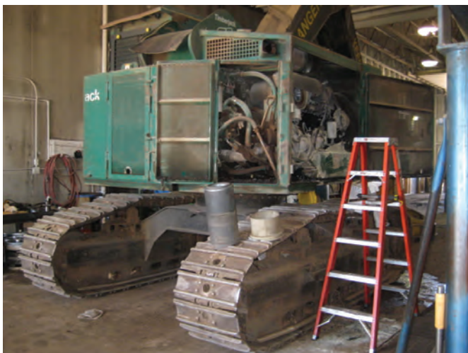
Fire damage occurred within the lower engine compartment on this feller buncher.
