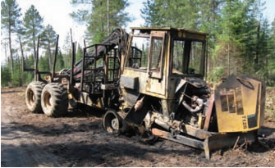
The forwarder from this incident after it was gutted by fire.
