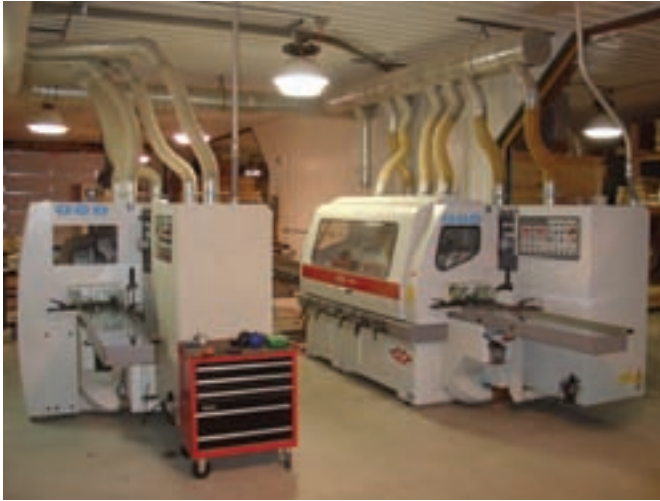
Two six-head molders used at East Dhu River.
