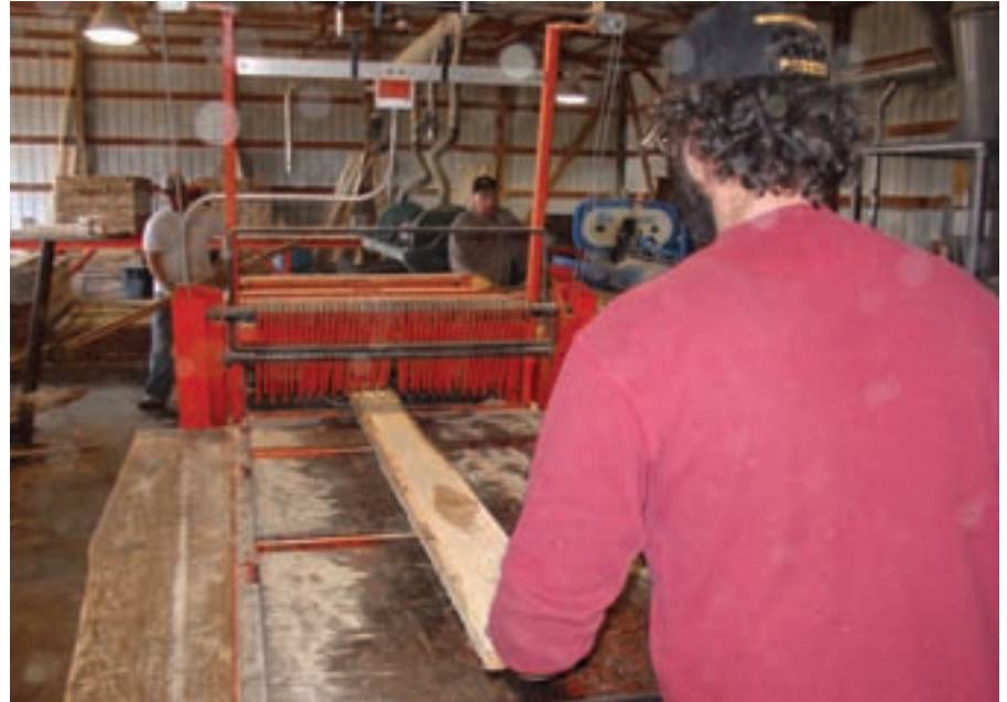
Brett Zadra feeds a board through the edger. B.A. Jacobsen (left) and Brett Kippola wait on the other end.
