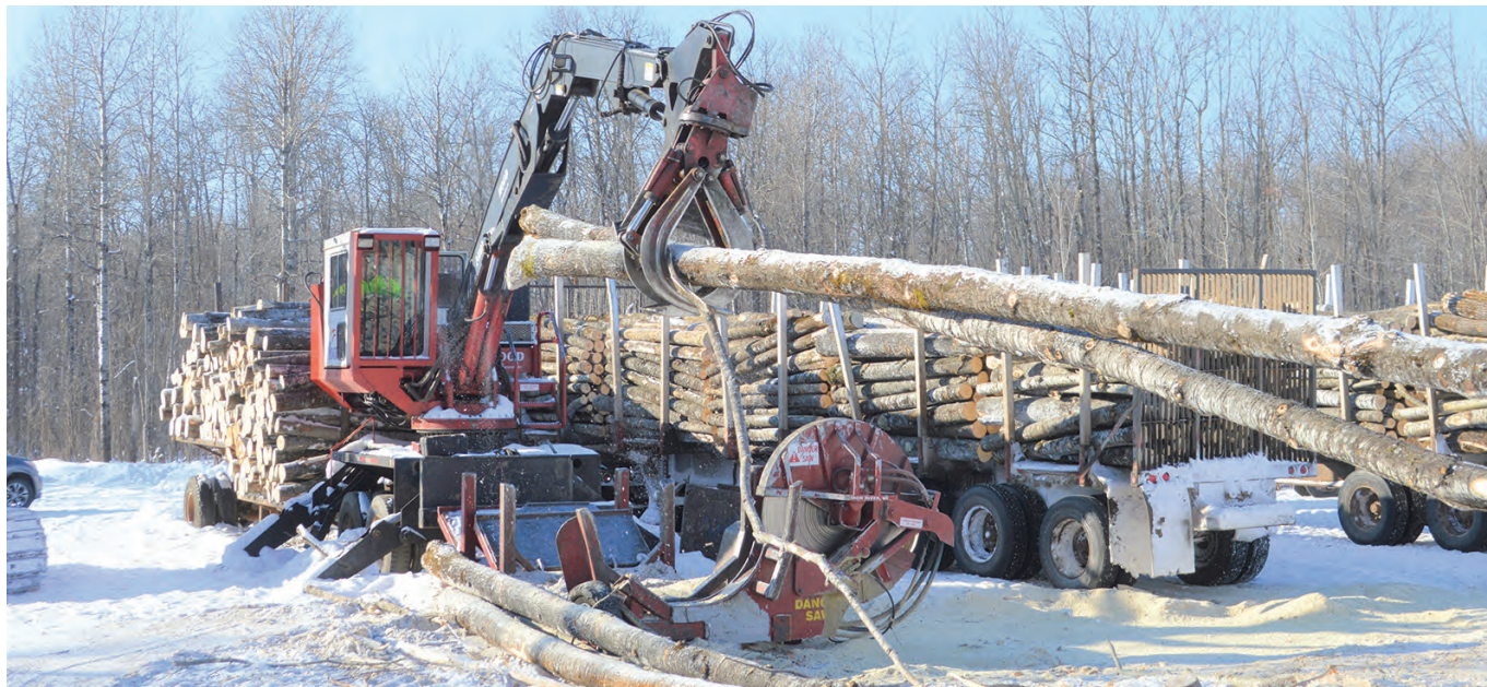
Nels Kimball III operates a Hood slasher/loader for Berthiaume Logging.
