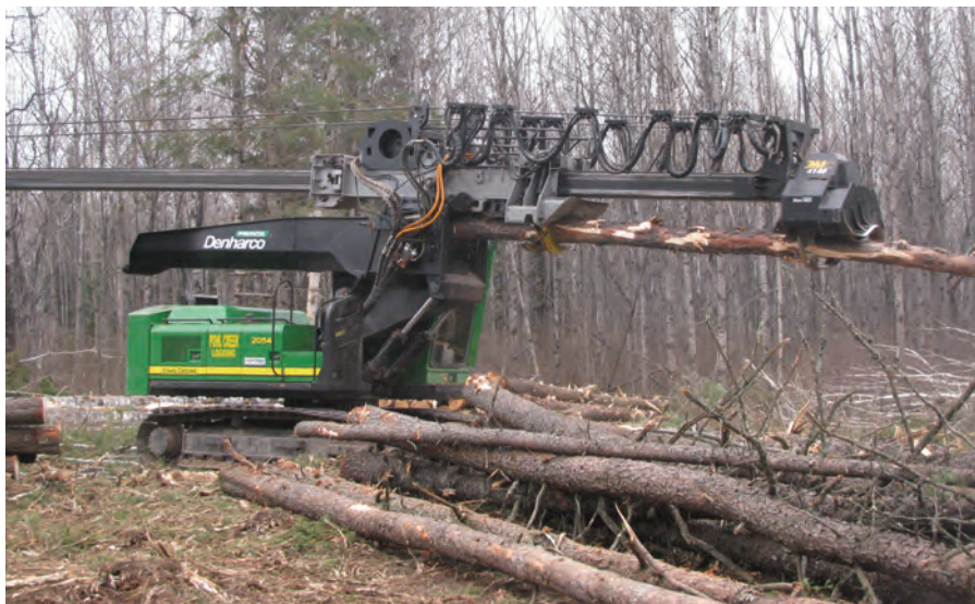
Pohl Creek Logging's delimber is a John Deere 2054 with a 4140 Denharco limbing head.
