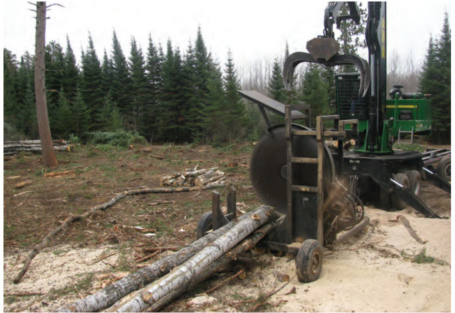
Pohl Creek's John Deere 437C knuckleboom loader has a HanFab 72 inch slasher.
