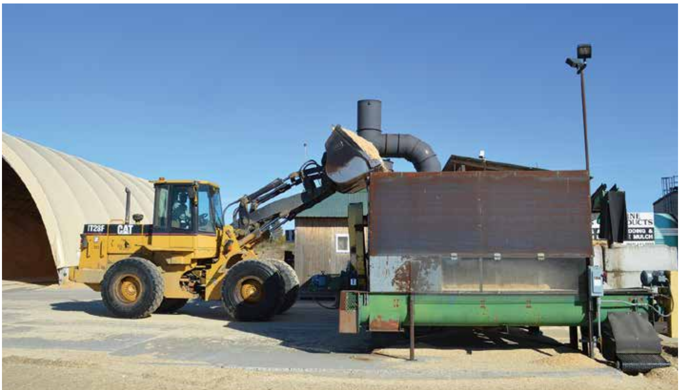
Green material for bedding is loaded into the feed box for processing at Pine Products' Bemidji facility.
