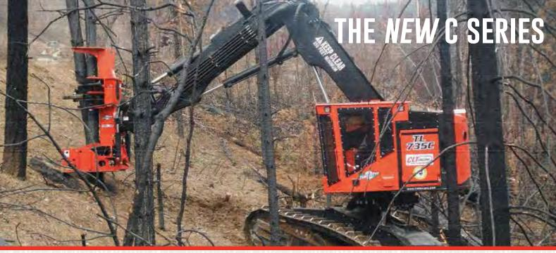
**THE NEW C SERIES FEATURES:** Hydrostatic swing, improved cab with taller windows, new style joystick pods, improved serviceability
