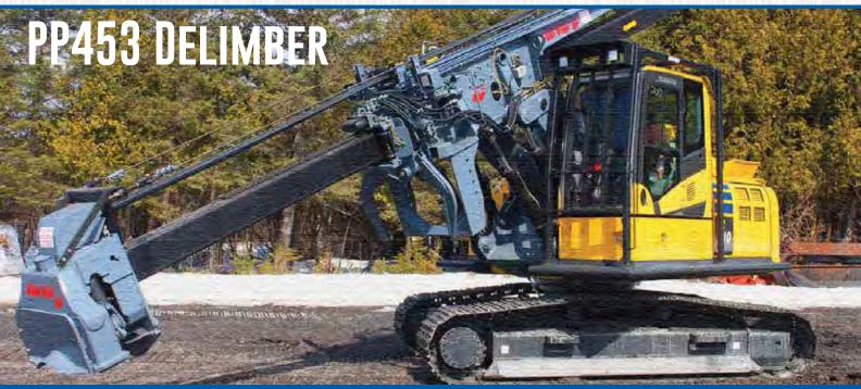
**PP453 FEATURES:** Versatile & durable, use with any type of topping system: twin topping knives, bar saw or circular saw
