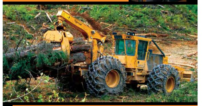
With Turnaround, the operator can comfortably drive the skidder blade-forward or grapple-forward while controlling all machine functions. In addition, the full infinite range of travel speeds and full maximum tractive effort are available in either direction at any engine speed, including low idle. No other skidder has these performance capabilities.
