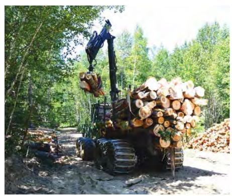
Scheff logging also operates three cut-to-length logging crews. Here, after aspen is harvested with a cut-to-length processor, a John Deere 1270D forwarder is used to pile the wood on the landing.
