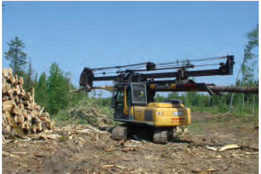
Troy Nelson operates the John Deere 200LC delimitter, equipped with a Lim-mit 2000B.
