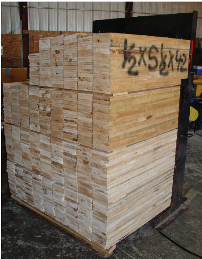
This bundle of finished pallet parts has been sawed to ½-inch by 5 ½ inches by 42 inches and is headed for a pallet maker in Brookings, South Dakota.
