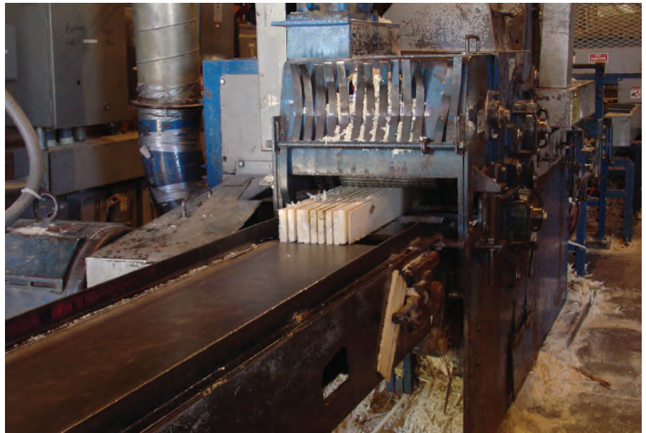
This Brewer RR resaw with a cant sizer has 32 blades. The slabs were pre-sawed before going through these bandsaws that cuts the wood to length and then to the desired thickness.
