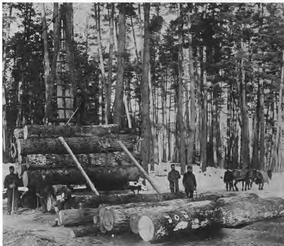
A typical horse-powered jammer; note the traveling block. A scaler works as the logs are loaded.
