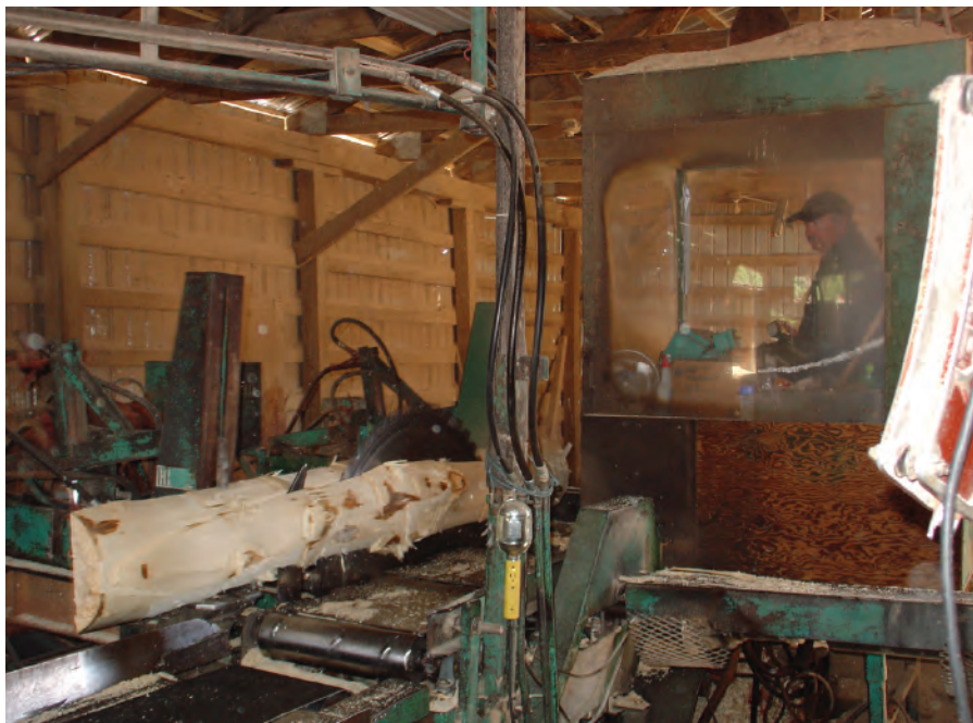
The log is sawed into slabs and cants before moving on to another line to be finished.
