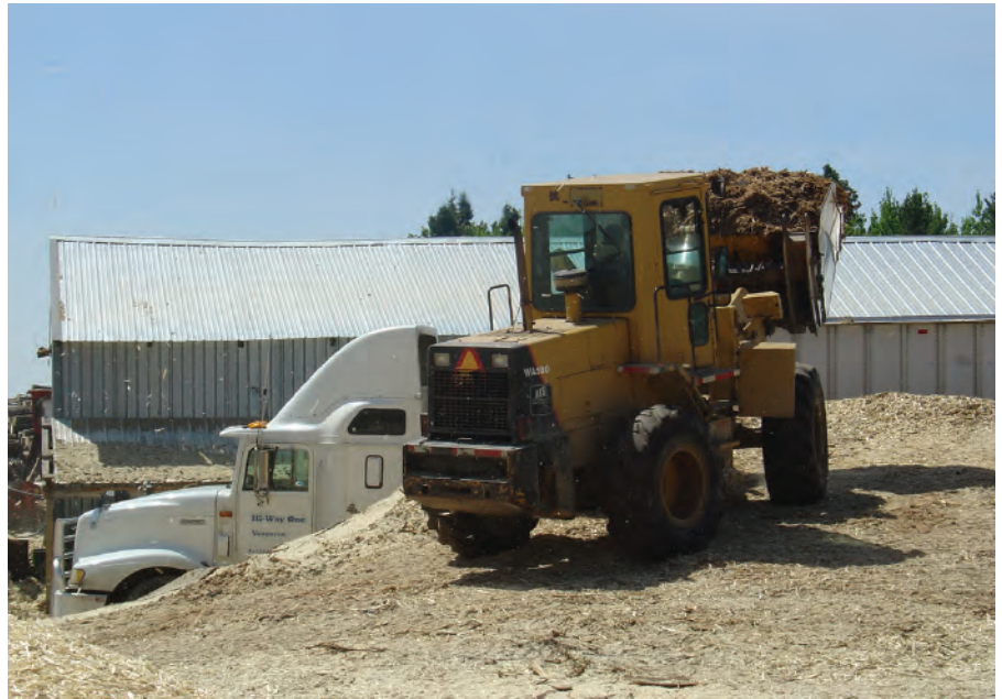
Residue is being loaded into a chip van to be hauled by Hi-Way One Ventures, the Petersons’ trucking company. The mill markets a variety of by-products, including sawdust, clean chips, and bark, for uses such as bedding, playground material, and boiler fuel.
