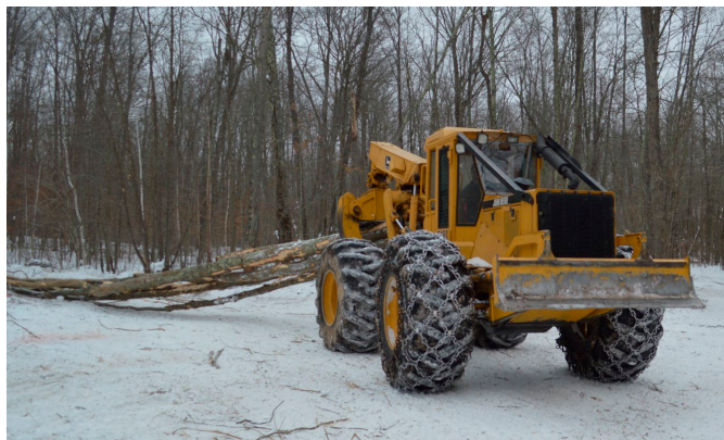
Vince Benson drags harvested oak from the delimeter to the landing with a John Deere 648G skidder. It’s one of two identical skidders working on this site, the other driven by Nate Benson.
