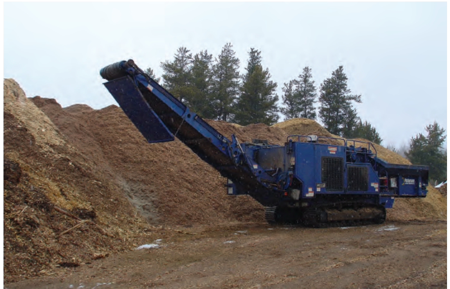
A Peterson Pacific grinder works on stockpiled wood outside the Walsh shop just north of Park Rapids. The biomass will be hauled to Boise in International Falls. The Walshes also utilize a Peterson "clean" chipper that removes bark, and also a Vermeer chipper.
