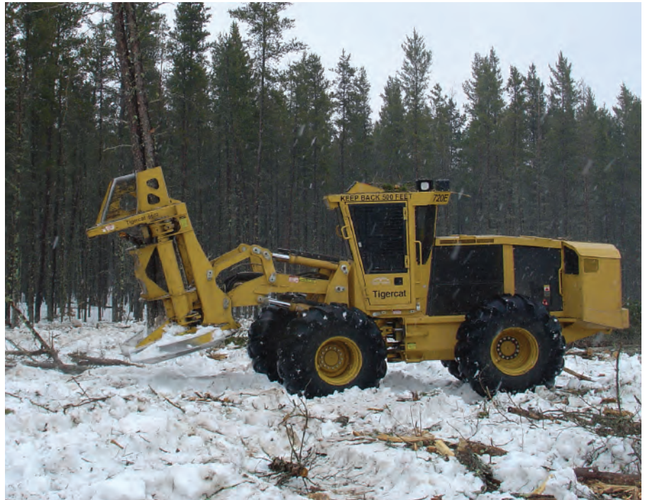
This Tigercat 720E feller buncher was one of three working on a clear-cut on a site near Badoura. The Walshes own four bunchers in all, including one with tracks. As far as other conventional logging equipment, the Walshes also own five skidders (one Tigercat and four John Deeres), two John Deere Delimiters, and a Tigercat loader with a Hanfab slasher.
