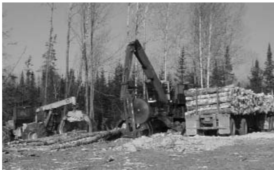
The skidder, slasher and truck on the landing, with nearly a full load.
