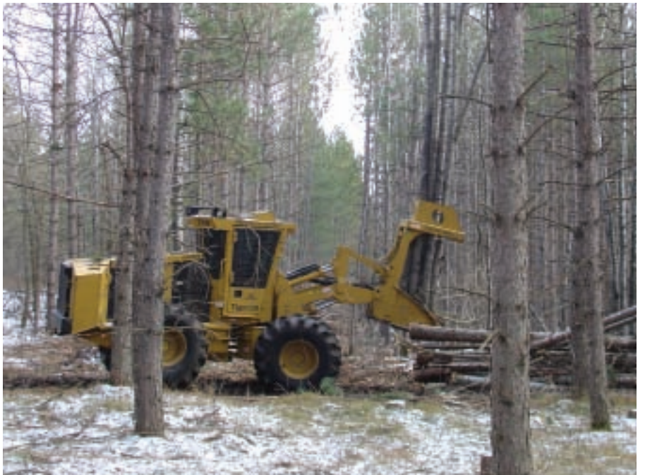
Smith's Tigercat shearer prepares to set down the trees he's just harvested. The shearer can hold up to half a dozen trees or more at a time.
