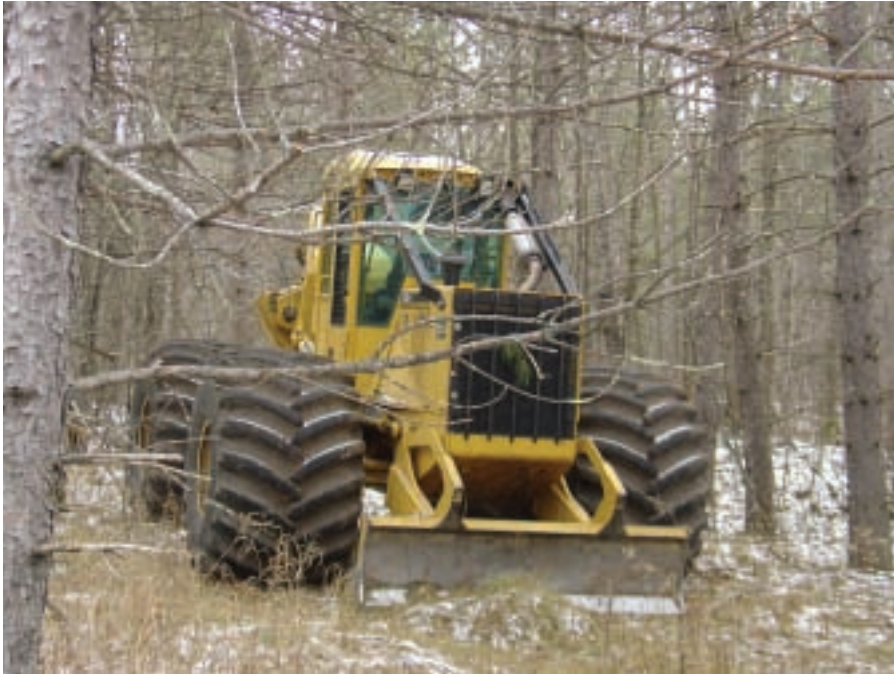
Smith's John Deere skidder. Once he's harvested the trees with the shearer, Smith skids them to the processor/loader.
