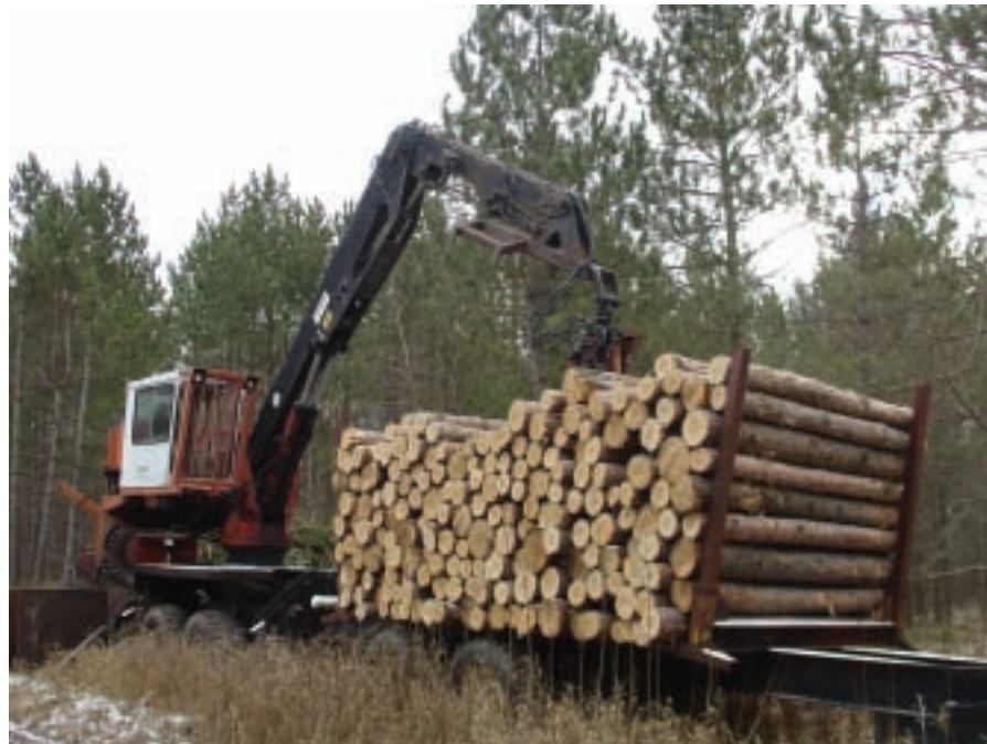
Smith's Hood loader is on an 8-wheel carrier. Immediately behind it is a Siiro processor.
