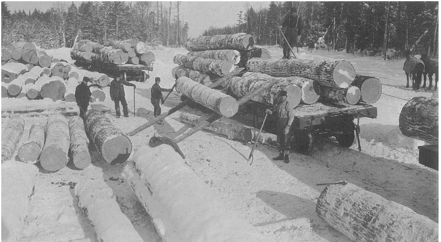
Cross haul loading was common in the early days. Horses furnished power to the cable which can be seen around the log half-way up on the skids. The man with cant hook was called a "sender-upper." He had to be skilled to make sure the log was "cut" at the right moment to land properly on the load. This was necessary where one end was bigger and thus traveled faster.
