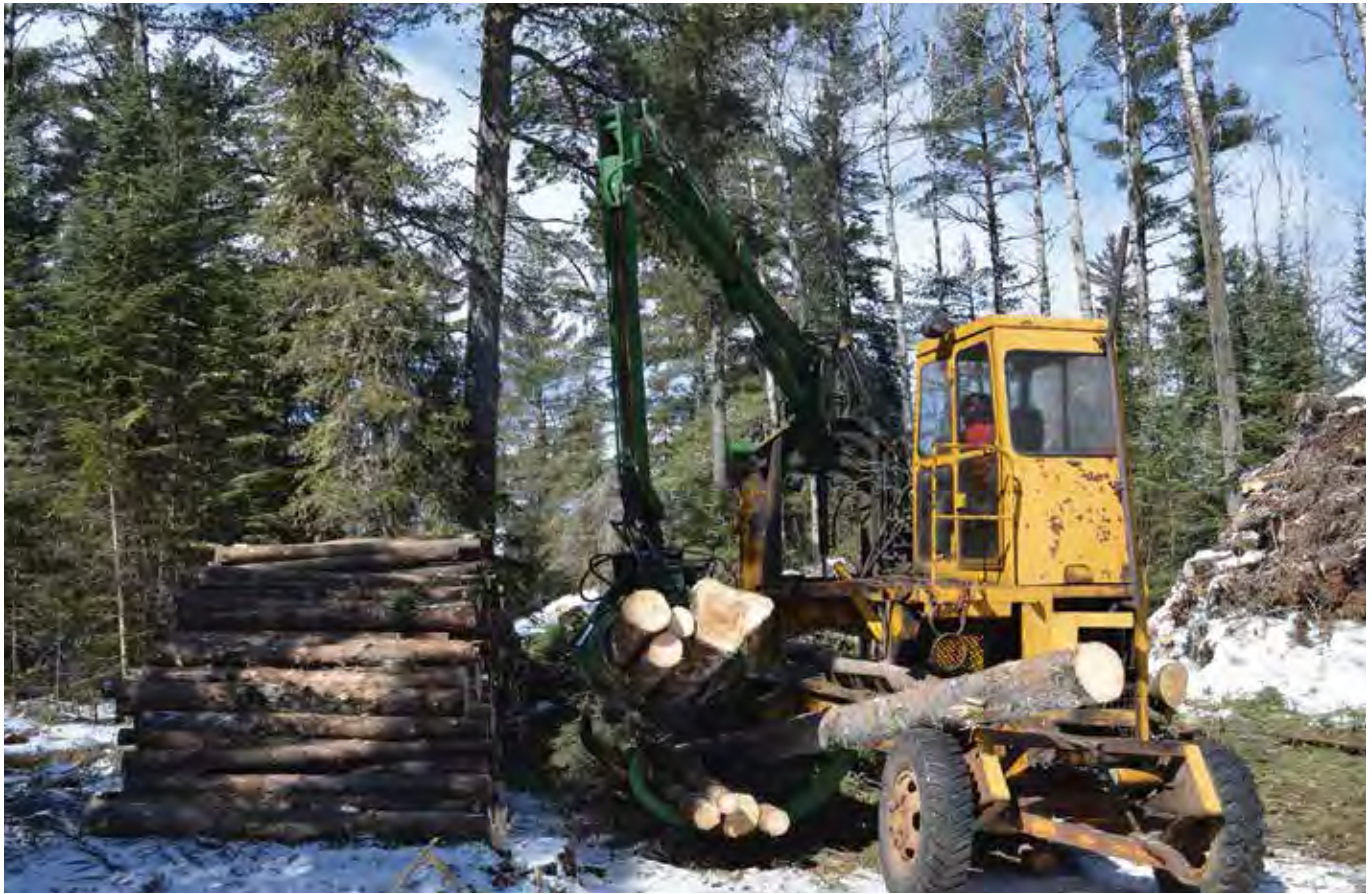
Hall loads processes the raw timber with a Can-Car processor, the predecessor to the Hahn Harvester. Only 38 of these machines were initially made. This one is number 19.
