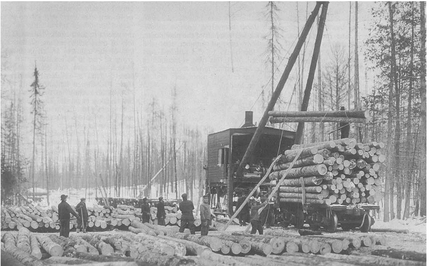
This is a steam-powered Clyde jammer. Empty cars – single-bunk Russells – are pulled under the jammer and then loaded. The picture shows two men on the left tailing down, two men are hookers and there's a top loader.
