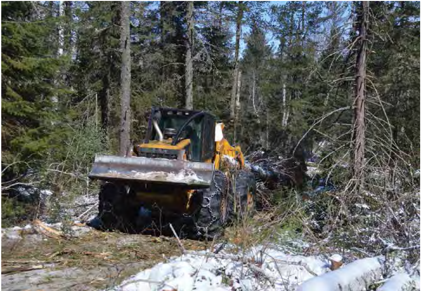
Hall utilizes a 1997 Cat 525 skidder to bring harvested timber to the landing for processing.
