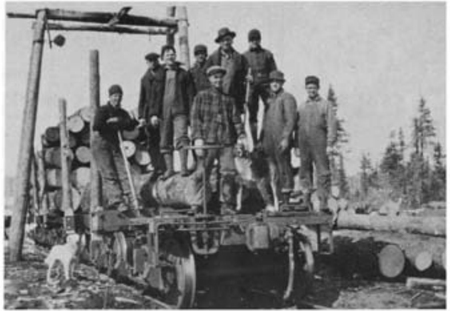
A small gypo camp skidding logs near Branson. Note the short Russell logger. Even the family dog got in the picture.
