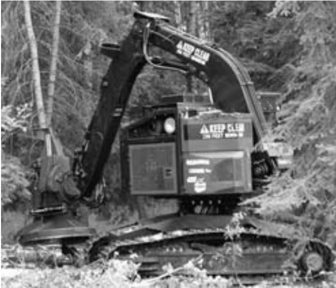
Denton Hasbargen operates the Timbco 425 feller buncher. Because of the terrain in the area, the Hasbargen's bunchers have tracks instead of tires.
