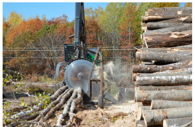
Chip Fletcher processes aspen with a John Deere 437E slasher/loader.
