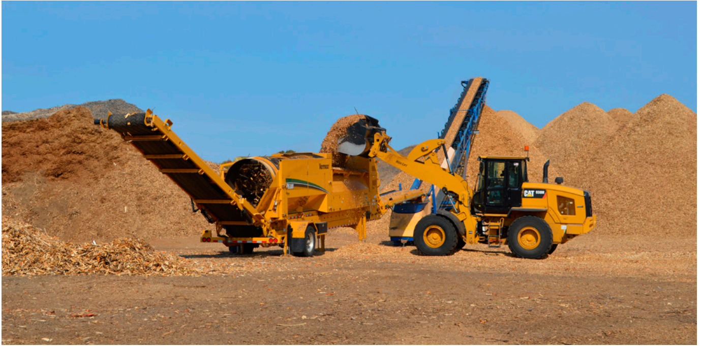
A Vermeer screener is loaded with chips at Fletcher Trucking's shop. Larger "overs" will be used for mulch, while turkey bedding will be made from the smaller material.
