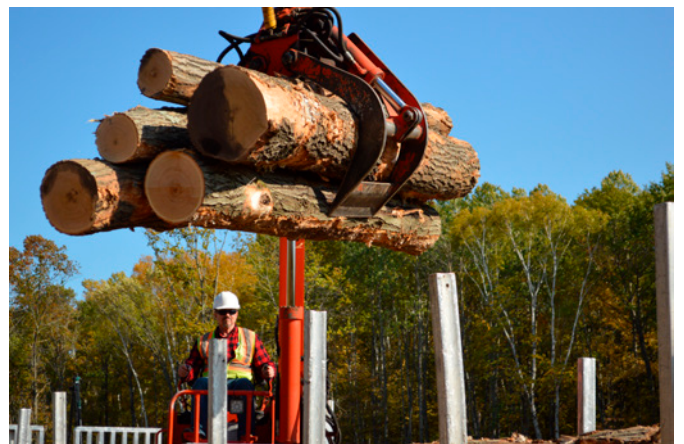
Driver Al Denny loads his truck with oak using a Serco 7500 center mount.
