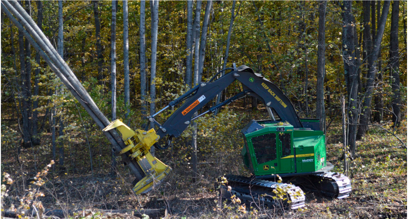
Zack Fletcher harvests aspen with a John Deere 853M feller buncher.
