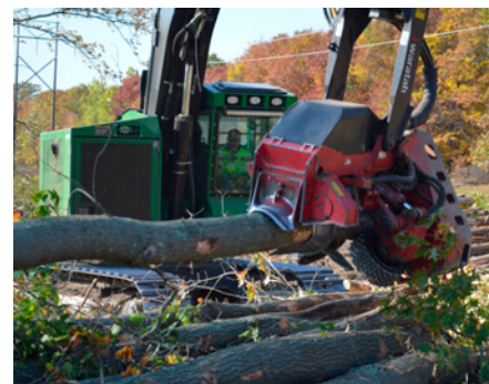
Shawn Fletcher took delivery on this John Deere 703JH cut-to-length processor two weeks ago. Here, he uses it to cut harvested oak to eight foot lengths.
