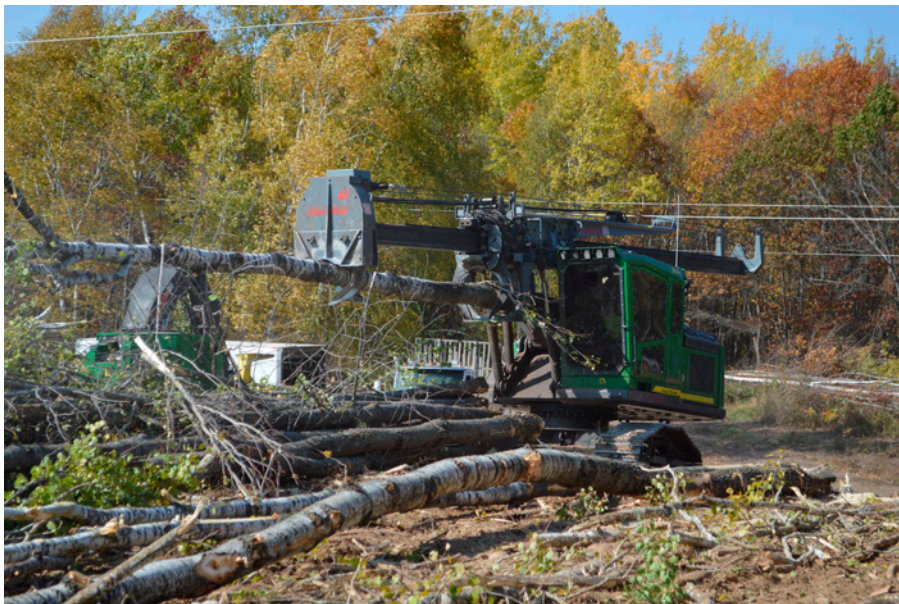
Aaron Schultz operates a John Deere 2154G stroke delimeter with a Pro Pac boom on Fletcher's Trucking's job northeast of Brainerd.
