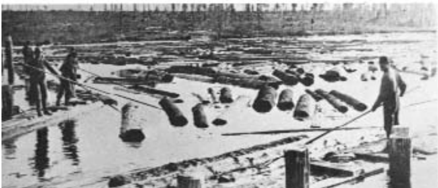
Logs scaled in the water at the spring works were scaled with a caliper.
