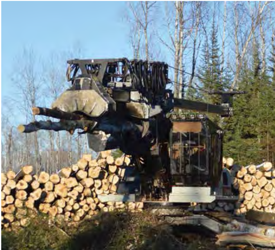
Brian Loughry operates a Link-Belt 210 delimer, with Denharco boom for Erickson Timber.
