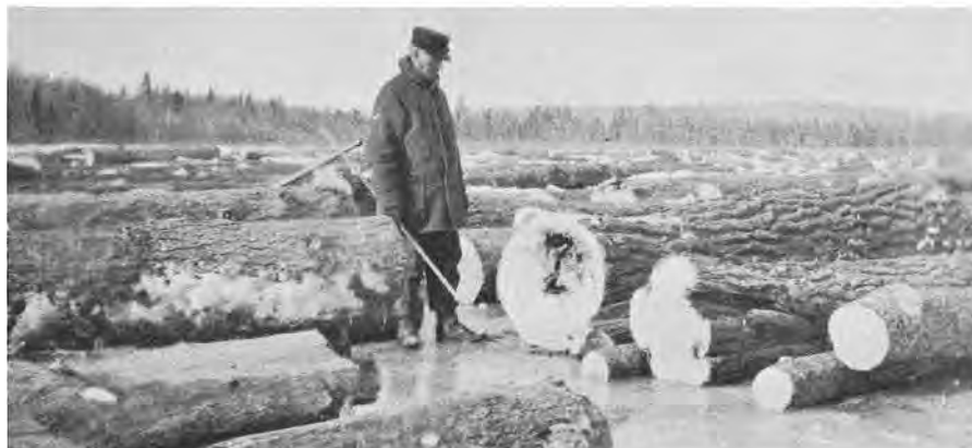
Logs scaled in the water at the sorting works were scaled with a caliper.
