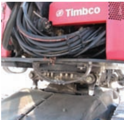
This is an example of additional steps added to mobile equipment for maintenance purposes.
