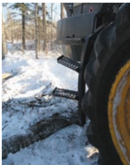
Steps in poor condition on mobile equipment may lead to problems.
