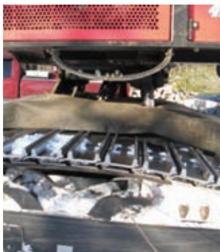
Another example of extra steps being added to mobile equipment to improve access and maintenance (both sides of machine).
