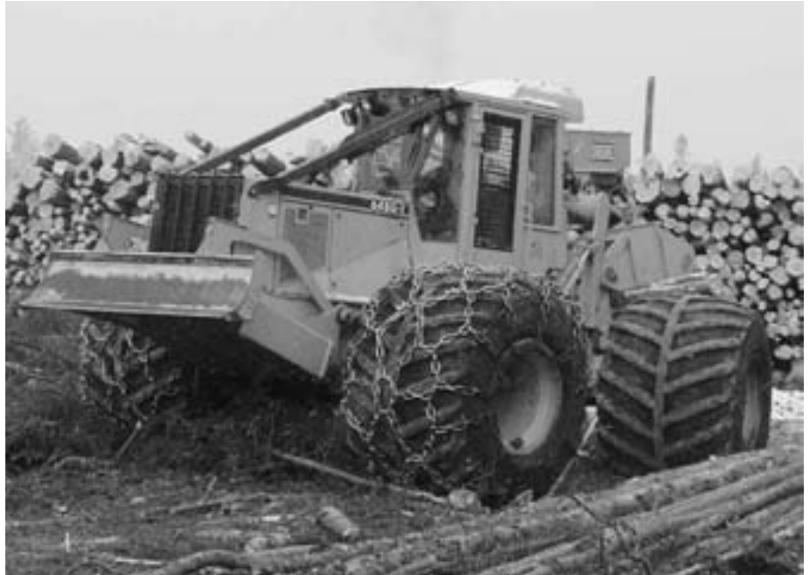
Ken Wendt needed to switch to this John Deere 648G skidder equipped with balloon tires because of soft ground conditions.
