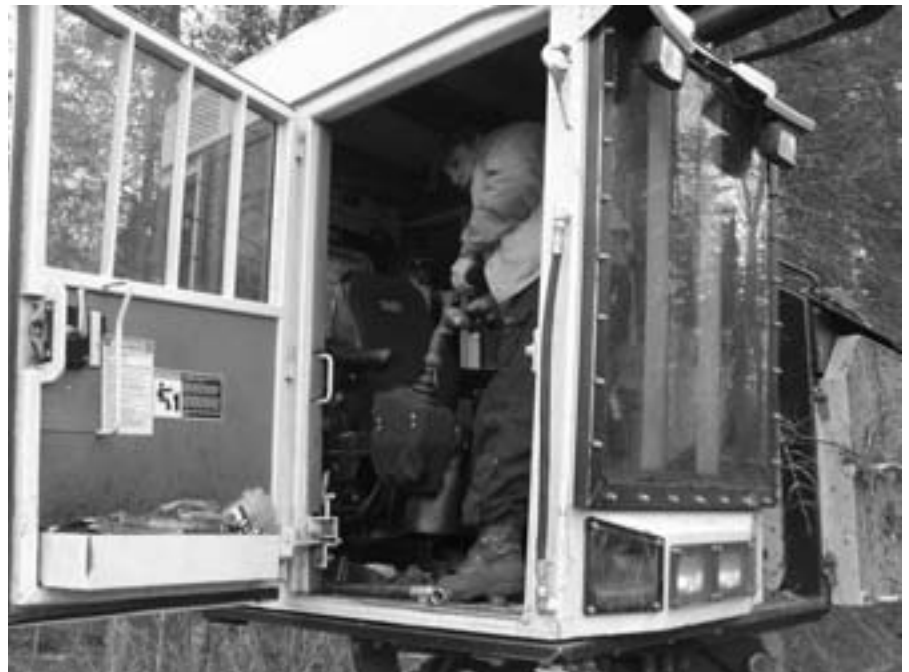
Denys Goychuk retrieves the time-motion recorder from Clarence Johnson's feller buncher. Goychuk visits the job site of each of the study participants every week to retrieve data. The process takes Goychuk about five minutes.
