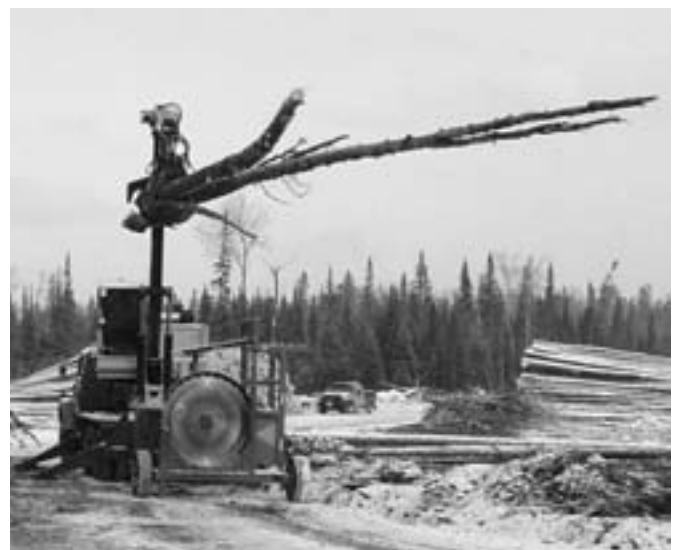
Ken Ziembra loads tree-length spruce onto a truck with a Barko 200D loader.
