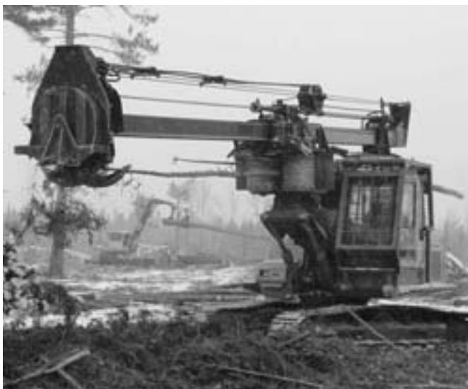
Curtis Street operates the John Deere 200LCL limber with a 2000B Lim-mit for Ziembra and Sons.
