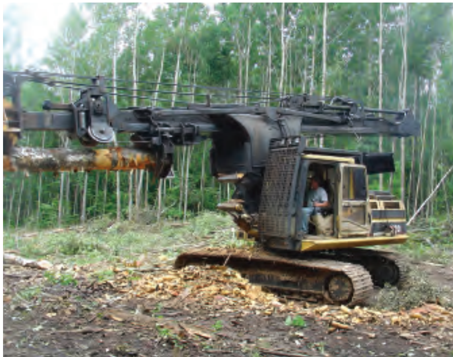
After skidding pulpwood to the landing, Habisch runs the Caterpillar 320 delimeter.
