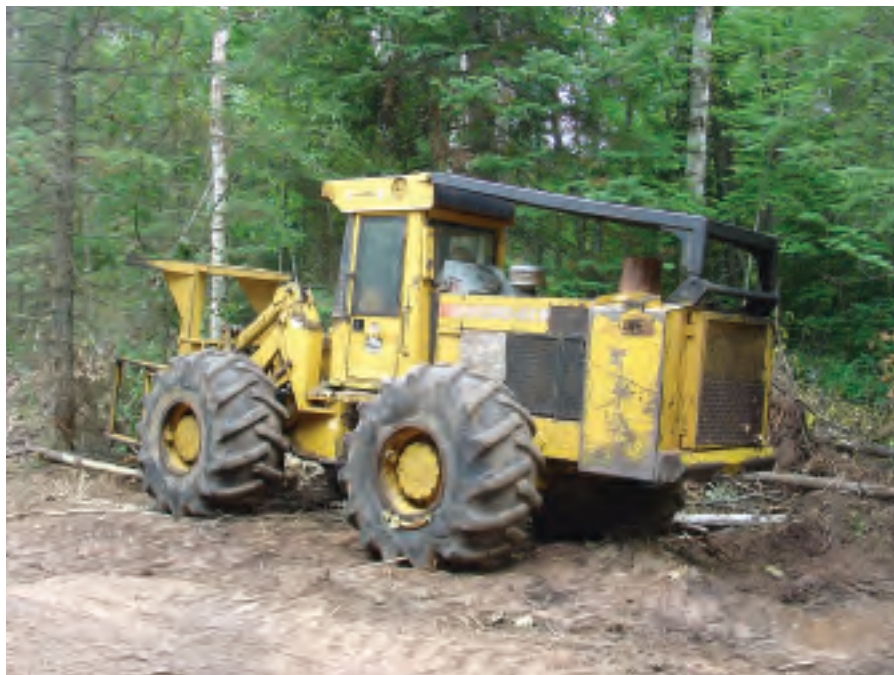
Simcoe and Habisch's Hydro-Ax 611 feller buncher sits on the landing, waiting to harvest more aspen, oak, and maple. With a two-man operation, Simcoe and Habisch can't operate all of the equipment at the same time.
