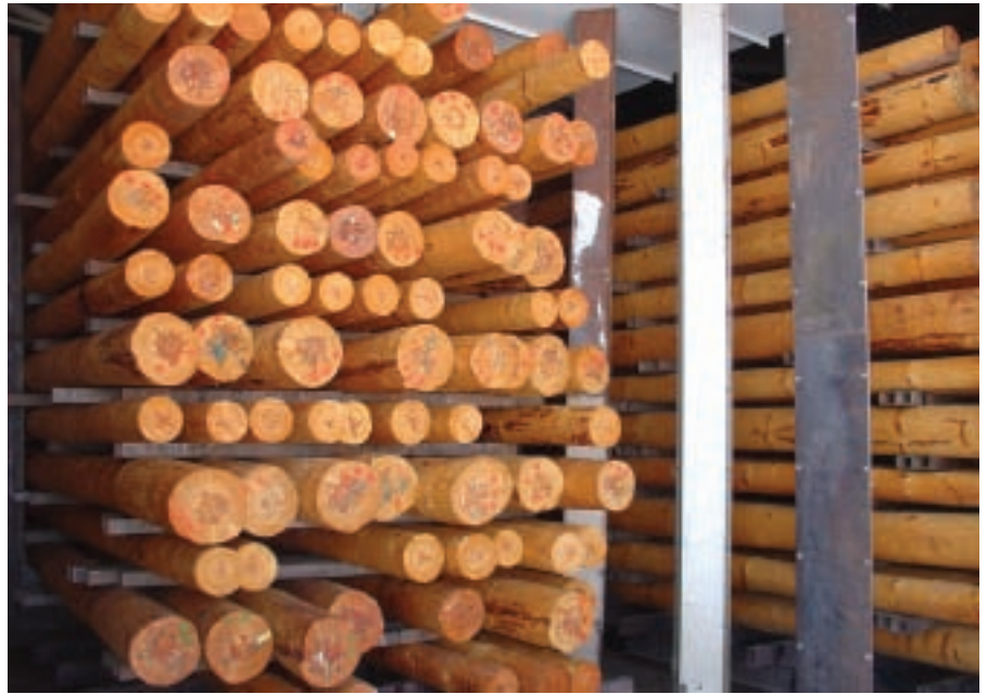
These red pine poles are seasoned and are ready to be removed by one of Bell's two kilns in Barron. One of the kilns just went on line in March and can handle up to 400 poles at a time. The other kiln can handle 550 poles. It takes three to six days to kiln dry the poles, depending on the temperatures used.
