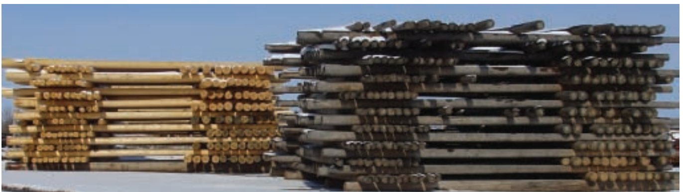
The air-seasoning process in Barron: the seasoning of the pile on the left is just starting while the pile on the right is completely seasoned.
