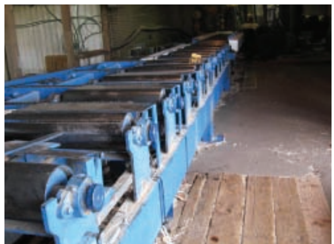
Walkway next to live roller deck
