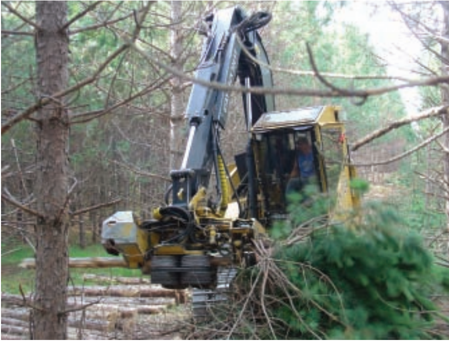
John Daniels operates the Fabtek FT133 Harvester. Daniels is cutting every fifth row and thinning within the other four rows to a basal area of 80 to 90.
