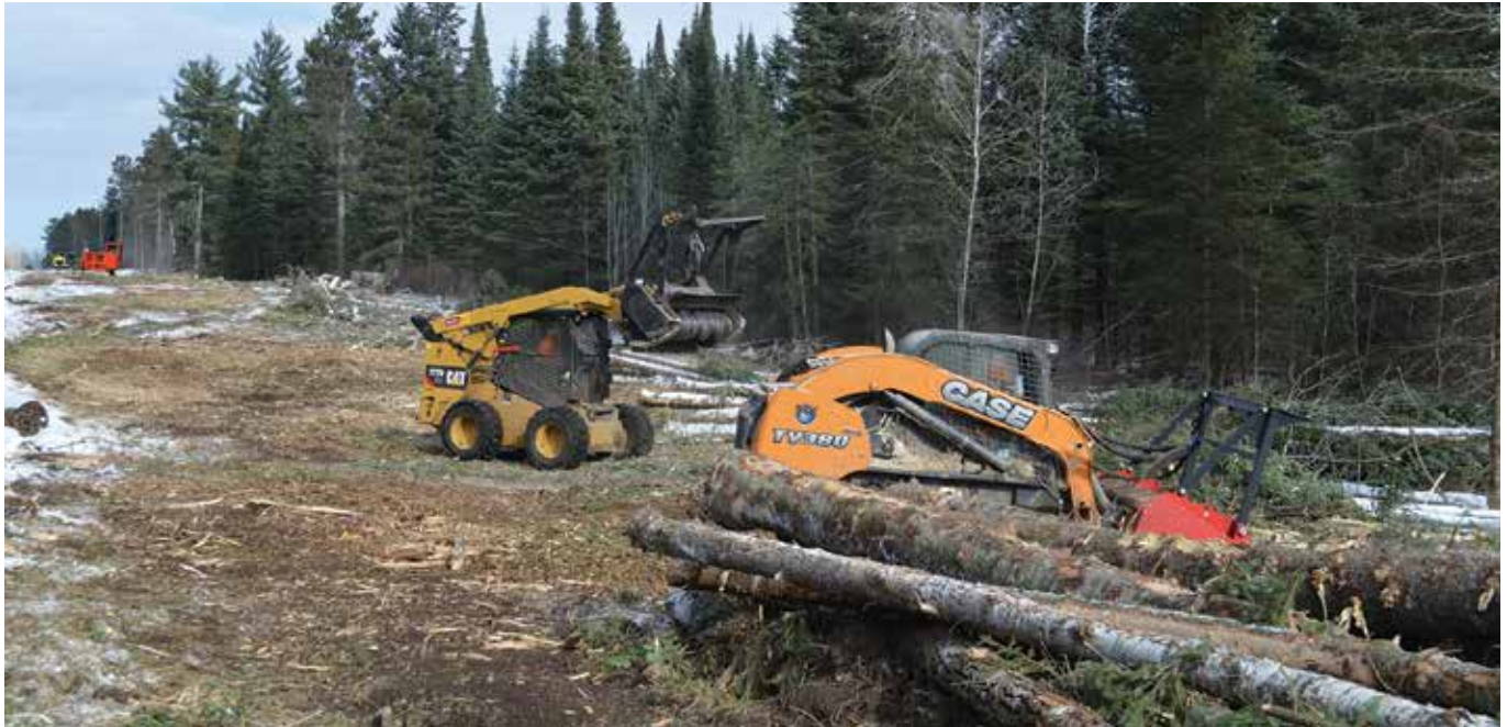
Bryan Hooker and Kurt DeMaris operate Case and Cat skid steers to mulch slash and stumps on the site. The Hookers say the skid steers are useful for landowners who like their pastures or fence lines brushed out, for folks with hiking or horse trails, or for deer hunters who like their shooting lanes cleared.
