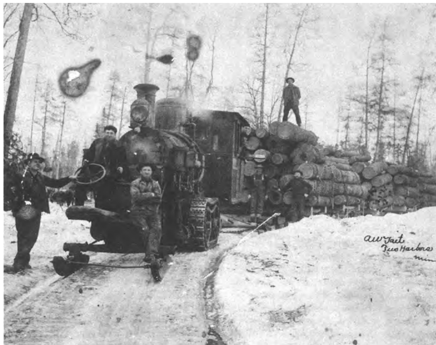
Below, top: a steam hauler of the Brooks-Scanlon line on a rutted ice road about 1903. Center: a four-horse team on a good ice road could pull three sleighs loaded with logs. Bottom: a typical four-horse team and loaded sleigh ready to move on an ice road.
