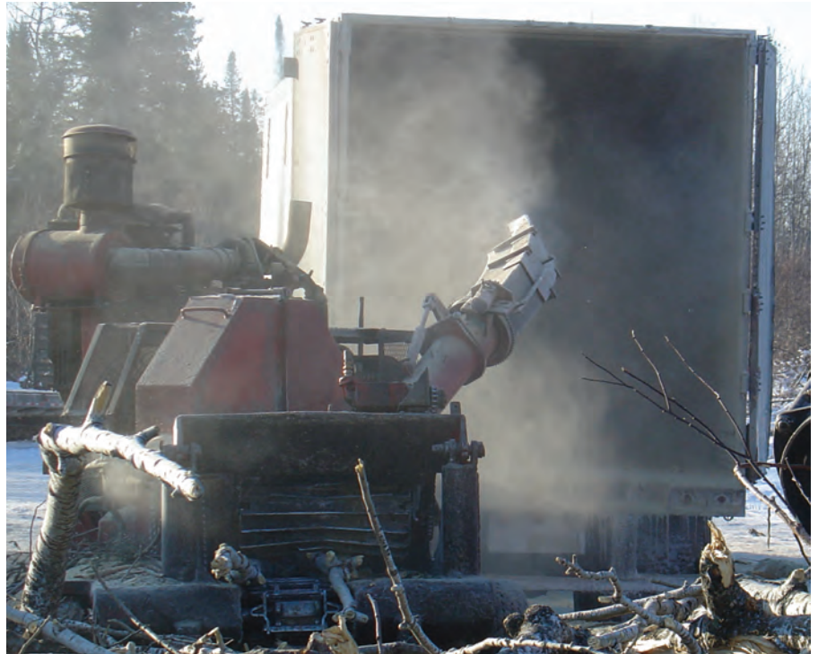
Tops and limbs are chipped and blown into Salmela’s chip van. This load will go to Sappi, one of a handful of mills that receive chips from Salmela
