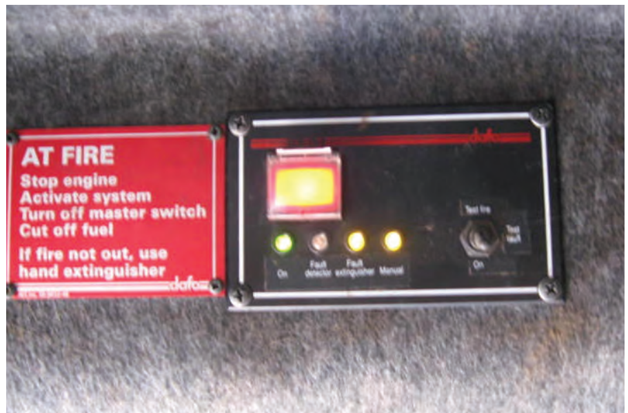
The manual control button for a fire self-suppression system.
