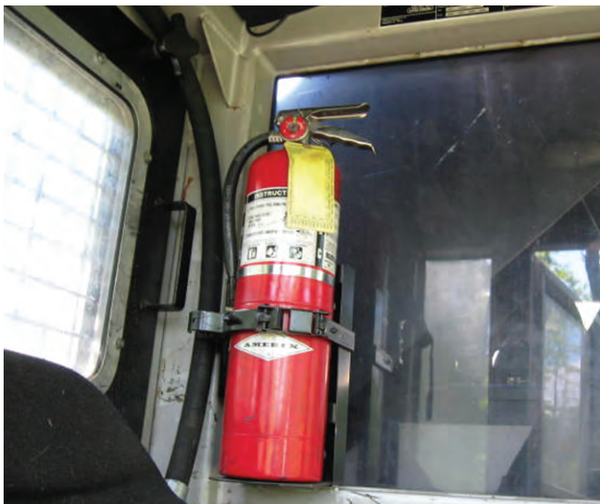
User-friendly, readily available fire extinguisher on a piece of mobile equipment.
