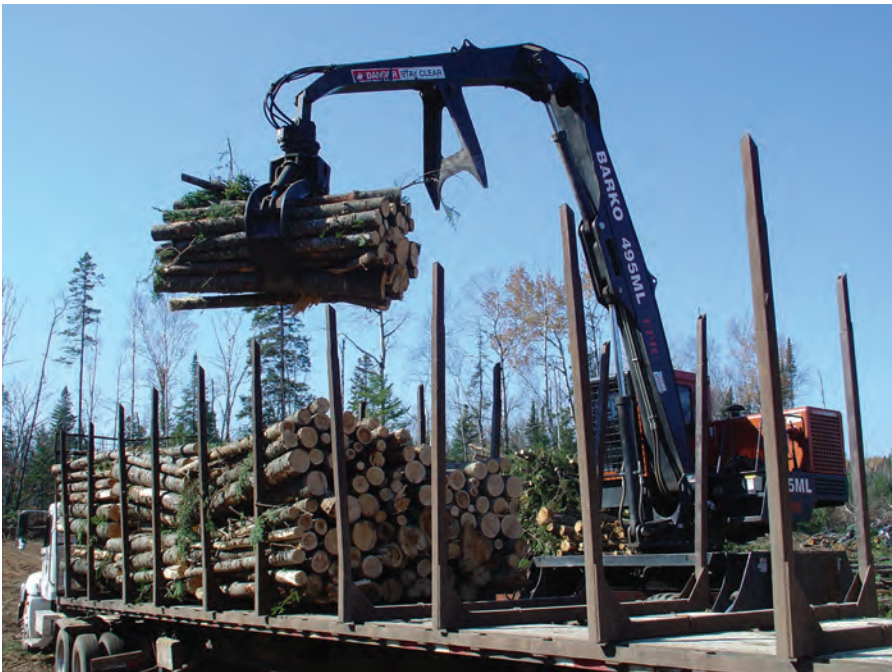
Rootkie runs the Barko 495ML Epic Loader/Slasher. He typically slashes after harvesting operations have been completed and the other equipment has moved to the next job.
