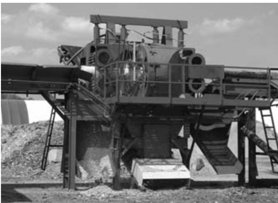
Raw timber is debarked and cut to length before it heads into the mill for finishing.
