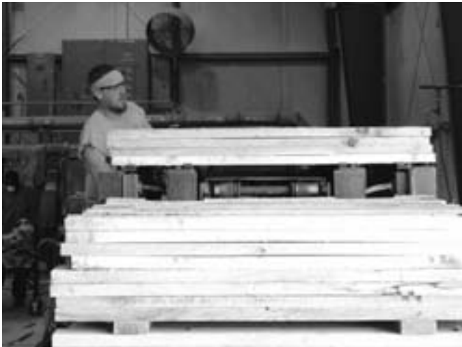
Scott Heyer stacks completed stringers.
