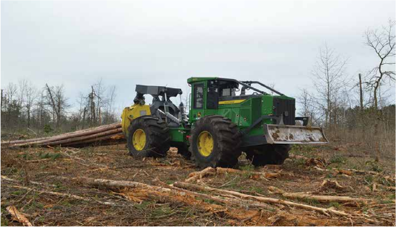
Harvested pine is dragged to the landing with a John Deere 848L skidder.
