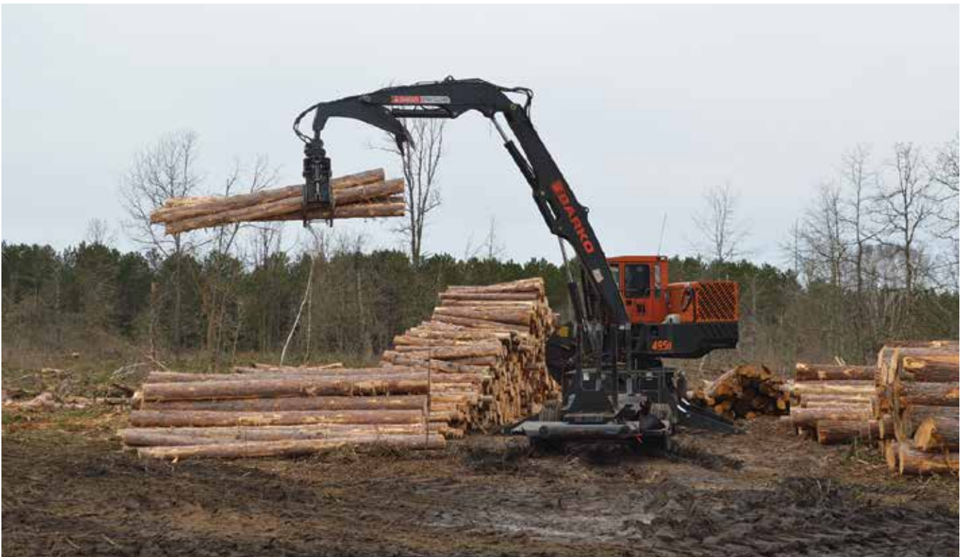
Pine is slashed into various lengths, depending on the wishes of the customer. Here, 16-foot lengths have been slashed and are being piled with a Barko 495B slasher/loader.
