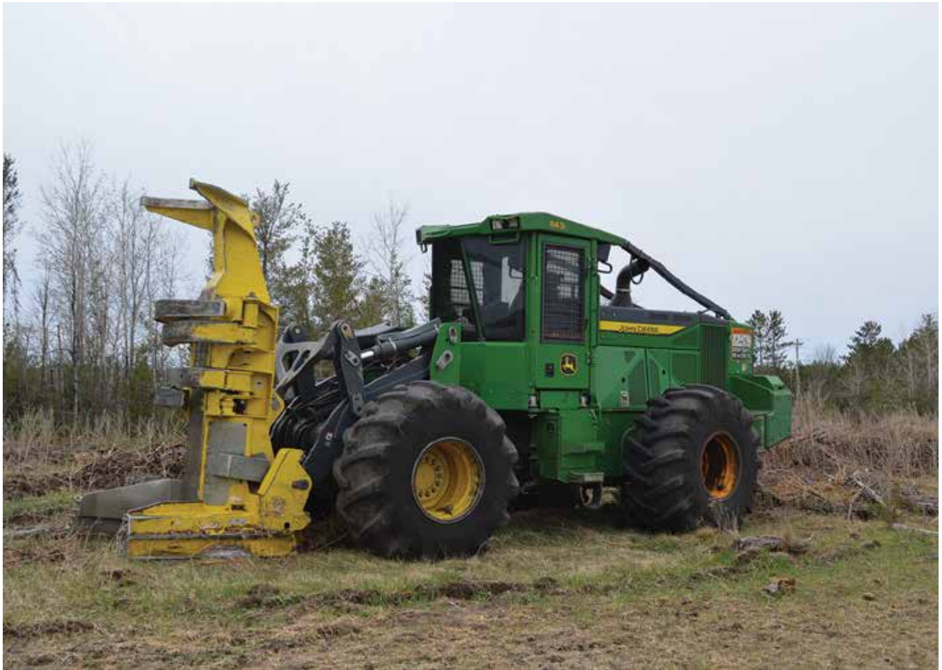
Edin Logging's John Deere 843L feller buncher features rubber tires rather than tracks.
