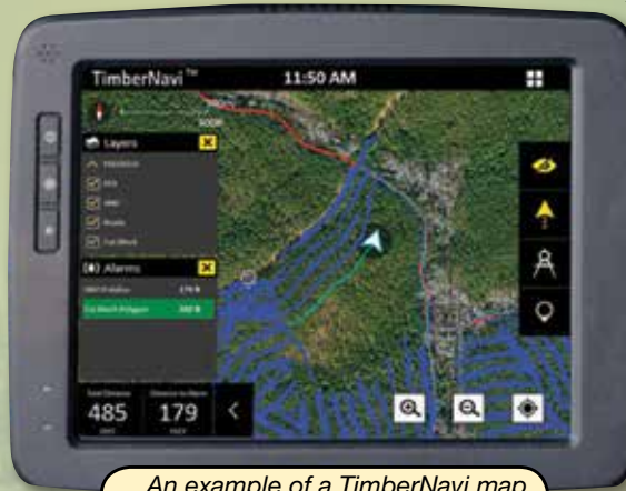
An example of a TimberNavi map that shows live positioning, cut block boundaries on a rugged monitor display inside the cab.
