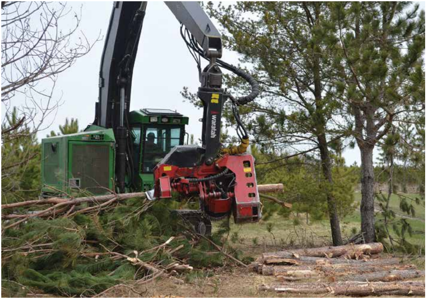
Marcus Edin uses a John Deere 703 cut-to-length processor with a 622B cutting head. The Edins use the processor for delimiting on the site. The wood is then forwarded to the landing with a John Deere 1010 single-bunk forwarder.
