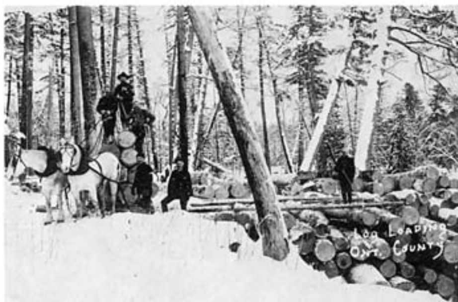
These logs were skidded to the river bank with a two-bank dory, then rolled off onto the bank. This type of dory could be used up to a half-mile haul.
