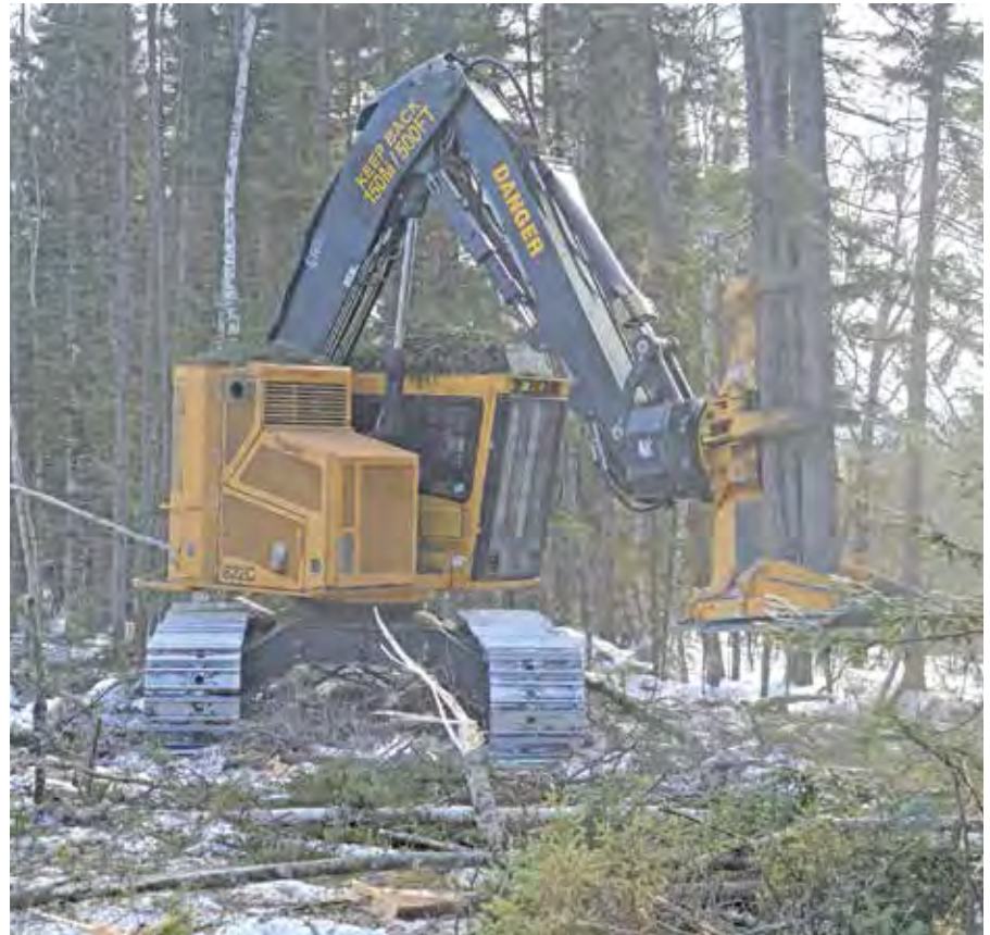
Jace Junker operates a Tigercat 822C feller buncher at the company’s logging job south of Littlefork.
