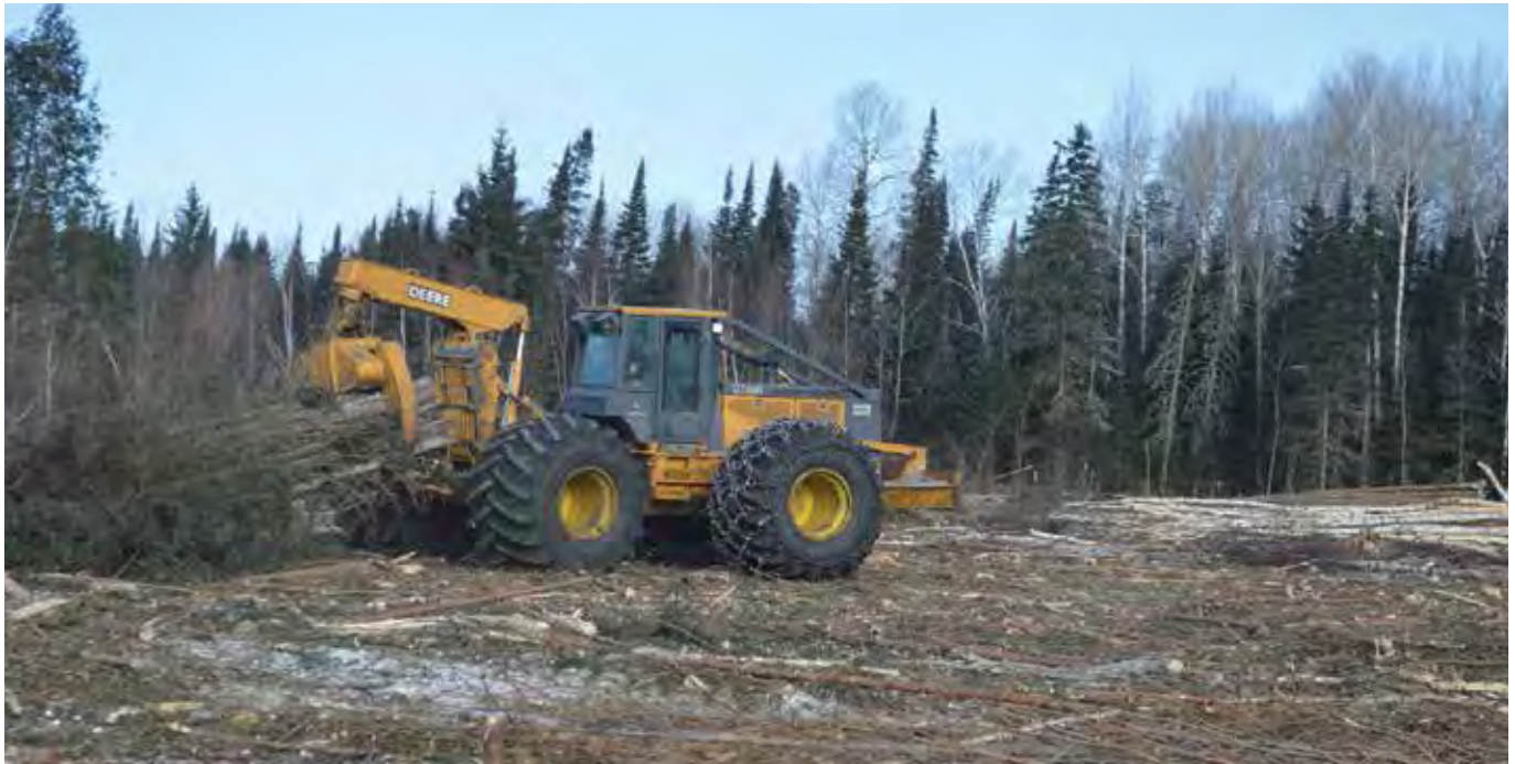
Nick Franko skids harvested tamarack to the landing in a John Deere 748G-III skidder.
