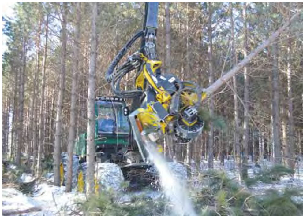
Kirk Smith operates a Timberjack 1270D cut-to-length harvester in a pine plantation.
