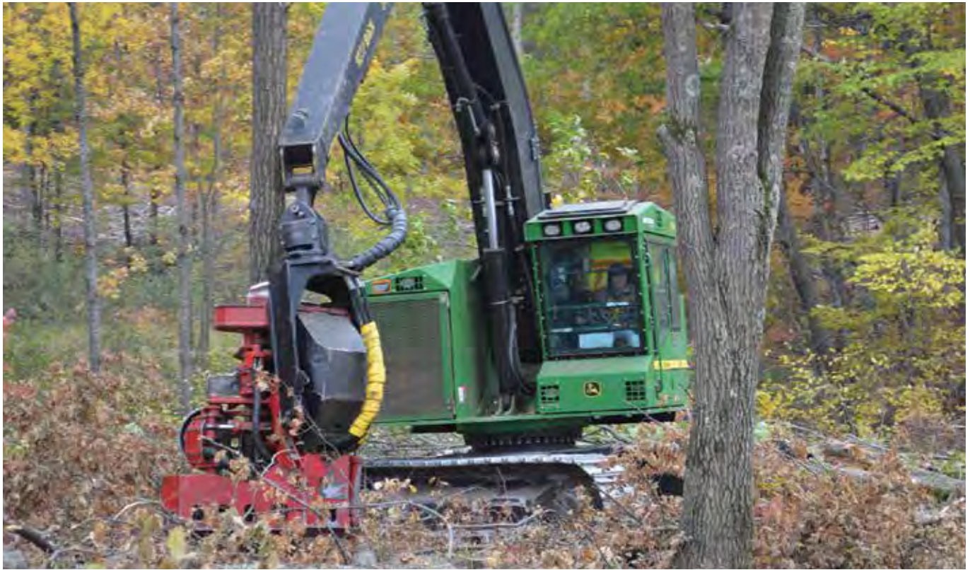
Alex Michalek operates M&M's John Deere 703JH Processor. The 703 has a larger cutting head which allows it to handle larger wood, and also offers more control in placing trees after they're harvested.
