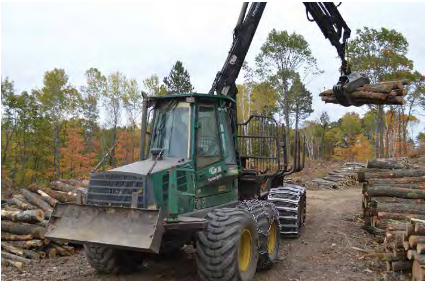
M&M Logging and Son utilizes two cut-to-length forwarders. Here, Dean Nestberg offloads harvested timber on the landing with a Timberjack 1110D.
