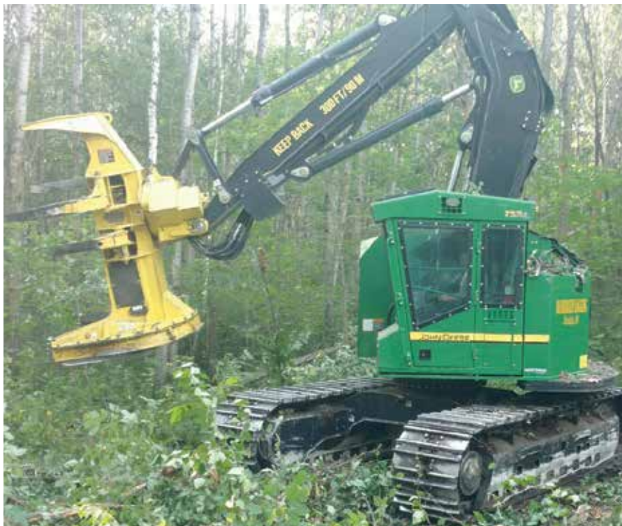
Hasbargen Logging has a mix of equipment, including this John Deere 753 tracked feller buncher.
