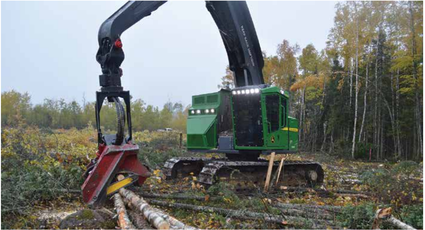
Jeff Sandnas operates the John Deere 803 processor, featuring a Waratah 622B cutting head. JATCO uses the machine to process wood at the stump, after it has been harvested.
