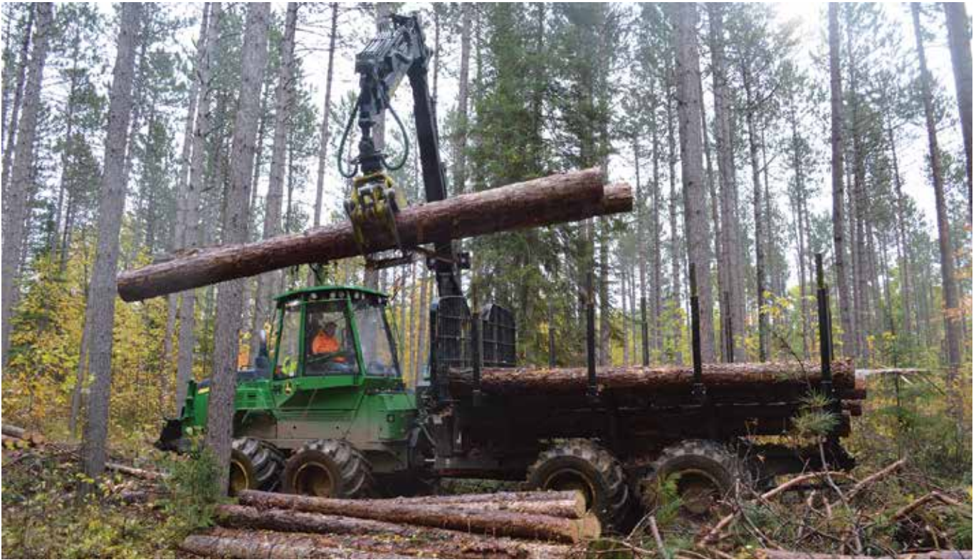
Rick Godden, Jr. operates the John Deere 1210G forwarder. JATCO purchased the 8-wheeled machine in January.
