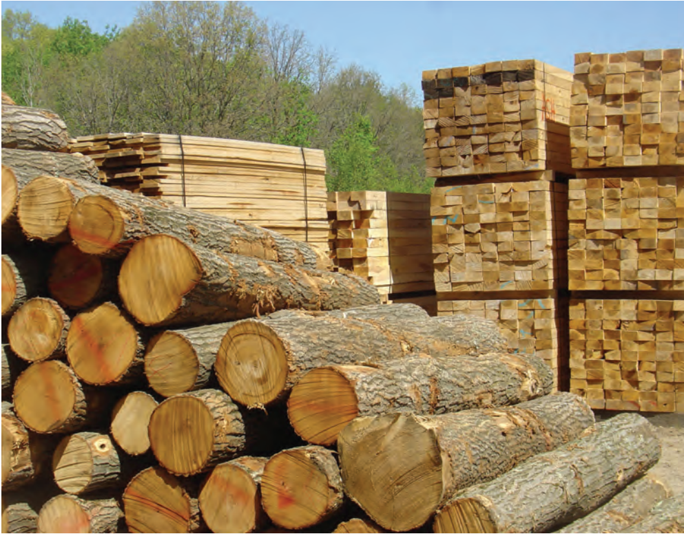
A pile of red oak logs wait to be sawed while finished timbers wait to be shipped. Nagel usually doesn't have to kiln-dry his product so it's generally shipped within a week of production.
