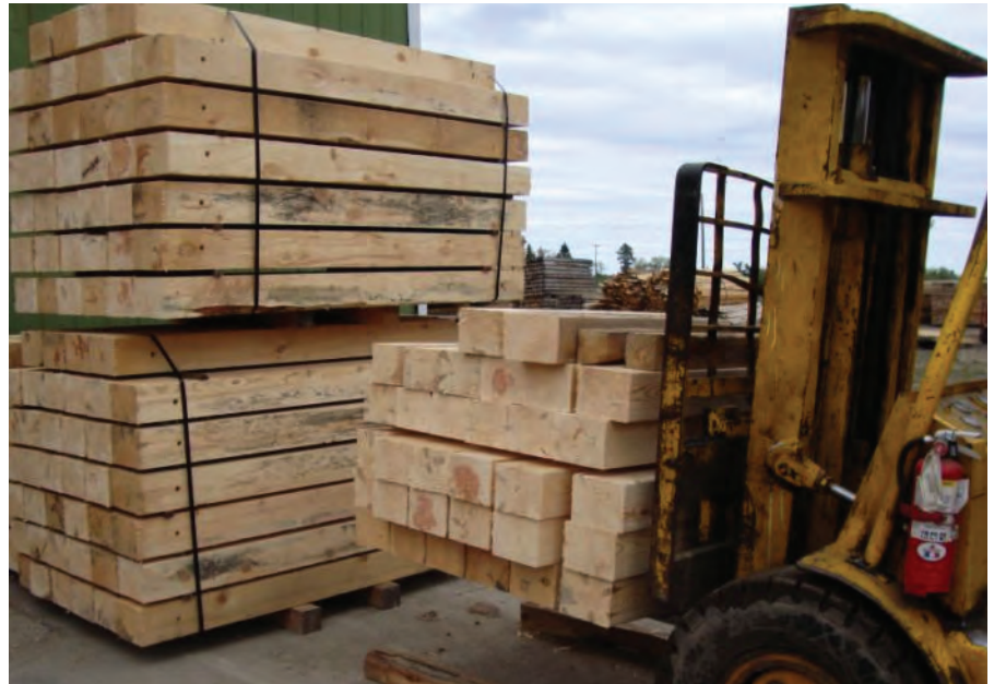
The space between the lumber pile and the loaded forklift was the pinch point in this situation.
