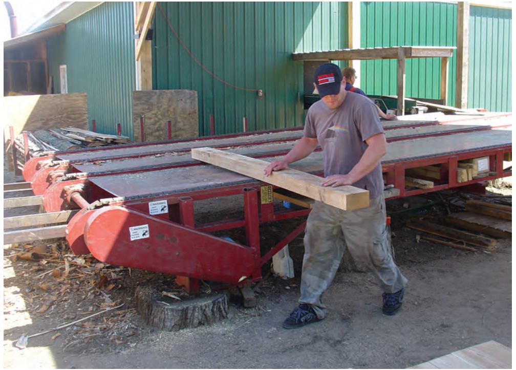
Mike Ratcliff sorts the sawed material into either pallet cants, railroad ties, or customized timbers for a variety of applications.
