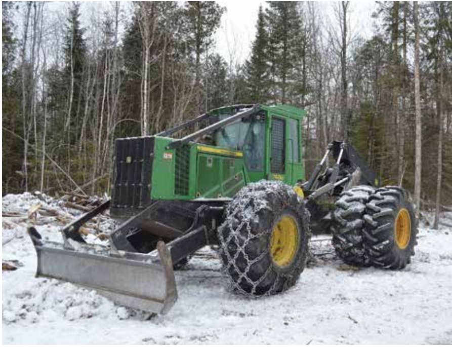
Pelland Logging utilizes dual tires on the back of this John Deere 748H skidder in order to be lighter on the ground, even in winter.
