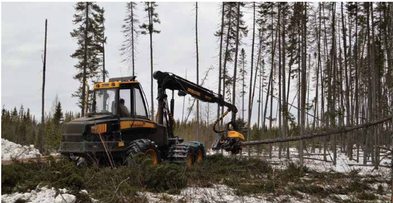
Gerald Jones works in black spruce with a newly purchased Ponsse Ergo cut-to-length processor.
