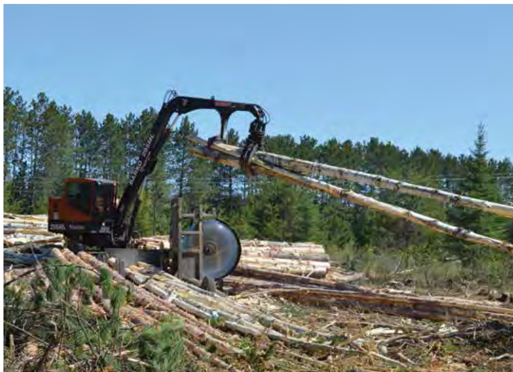
Harvested aspen is slashed and loaded by Cory Korba, with a Barko 295ML slasher.
