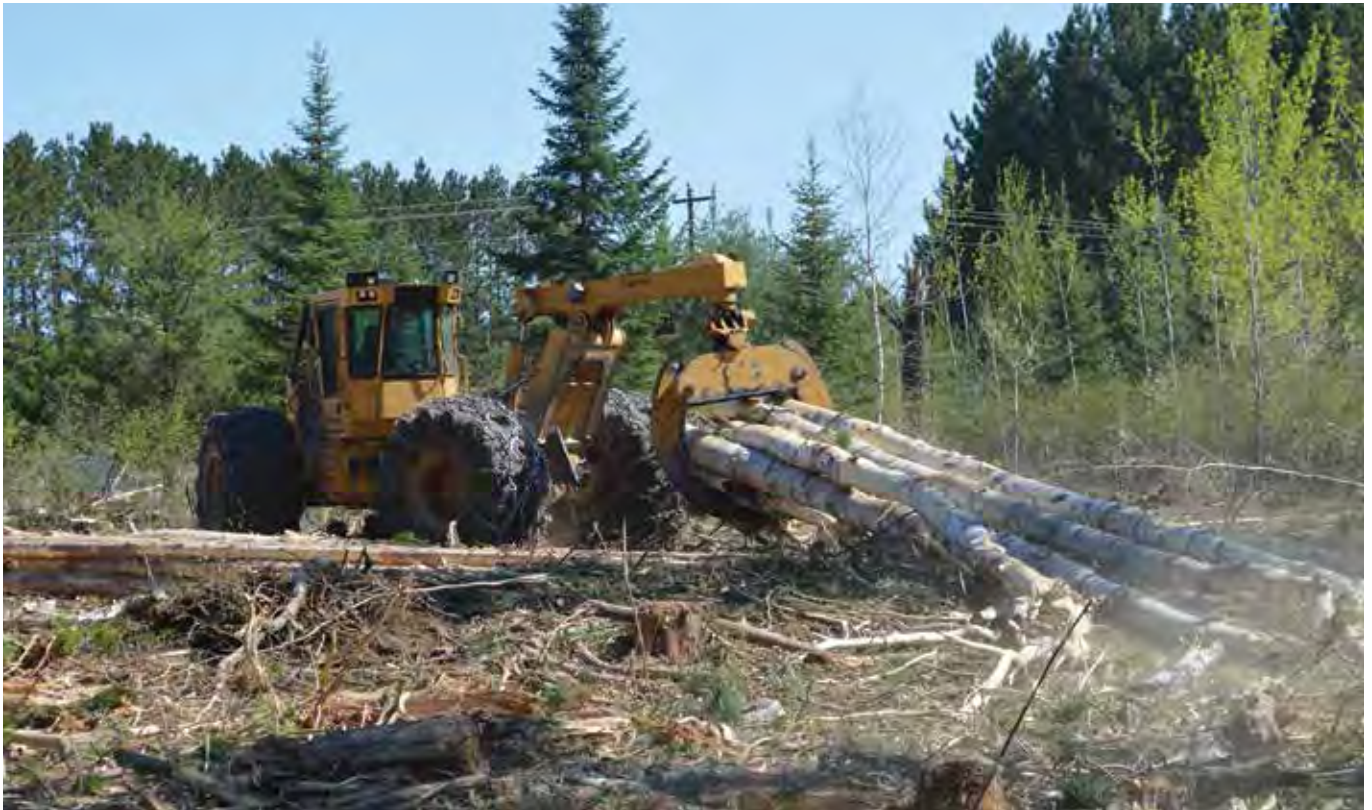
Bob Stecker drags harvested aspen to the landing with a Tigercat 610C skidder. It's one of four skidders Hustad utilizes on his logging sites.
