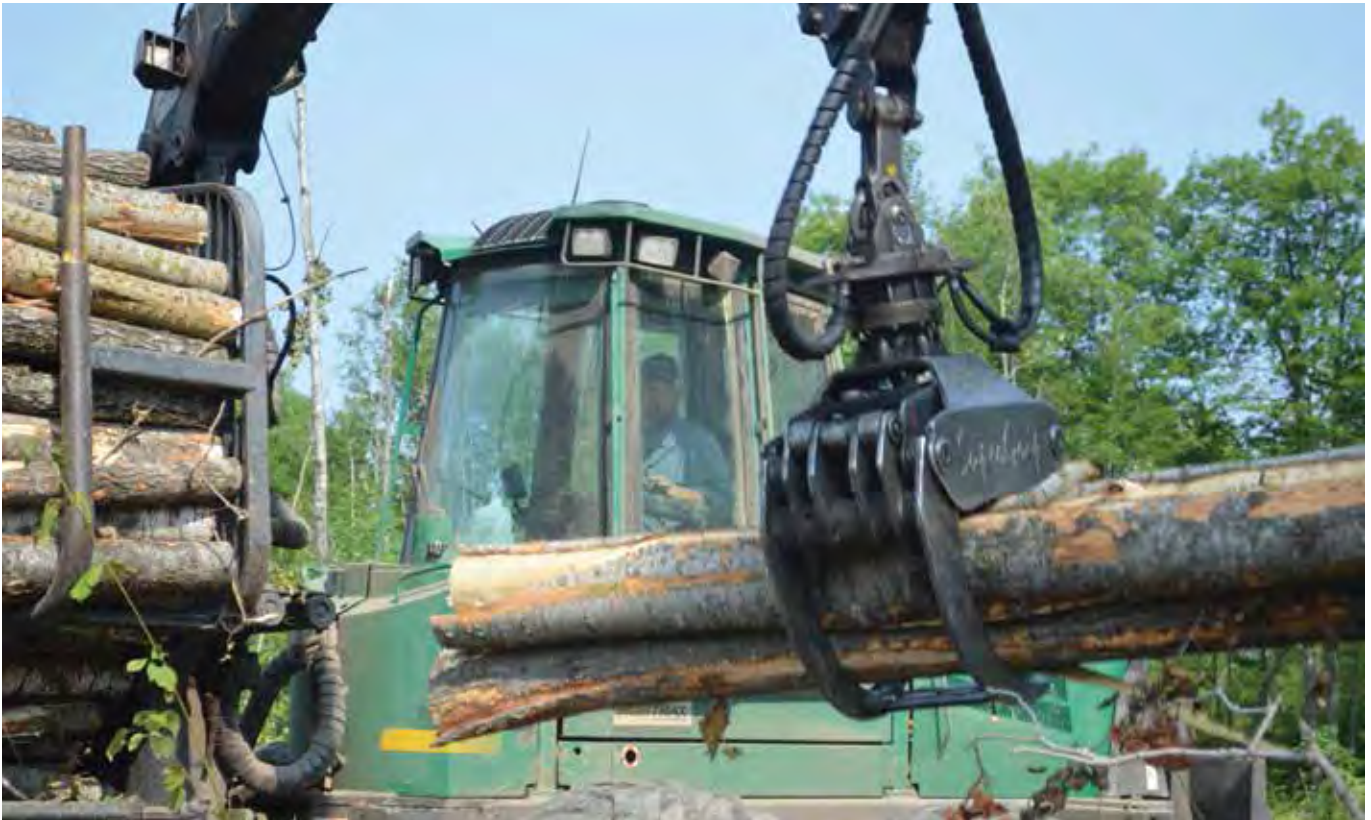
Ron Beckman, Jr. watches as he loads aspen onto his Timberjack 1110D forwarder.
