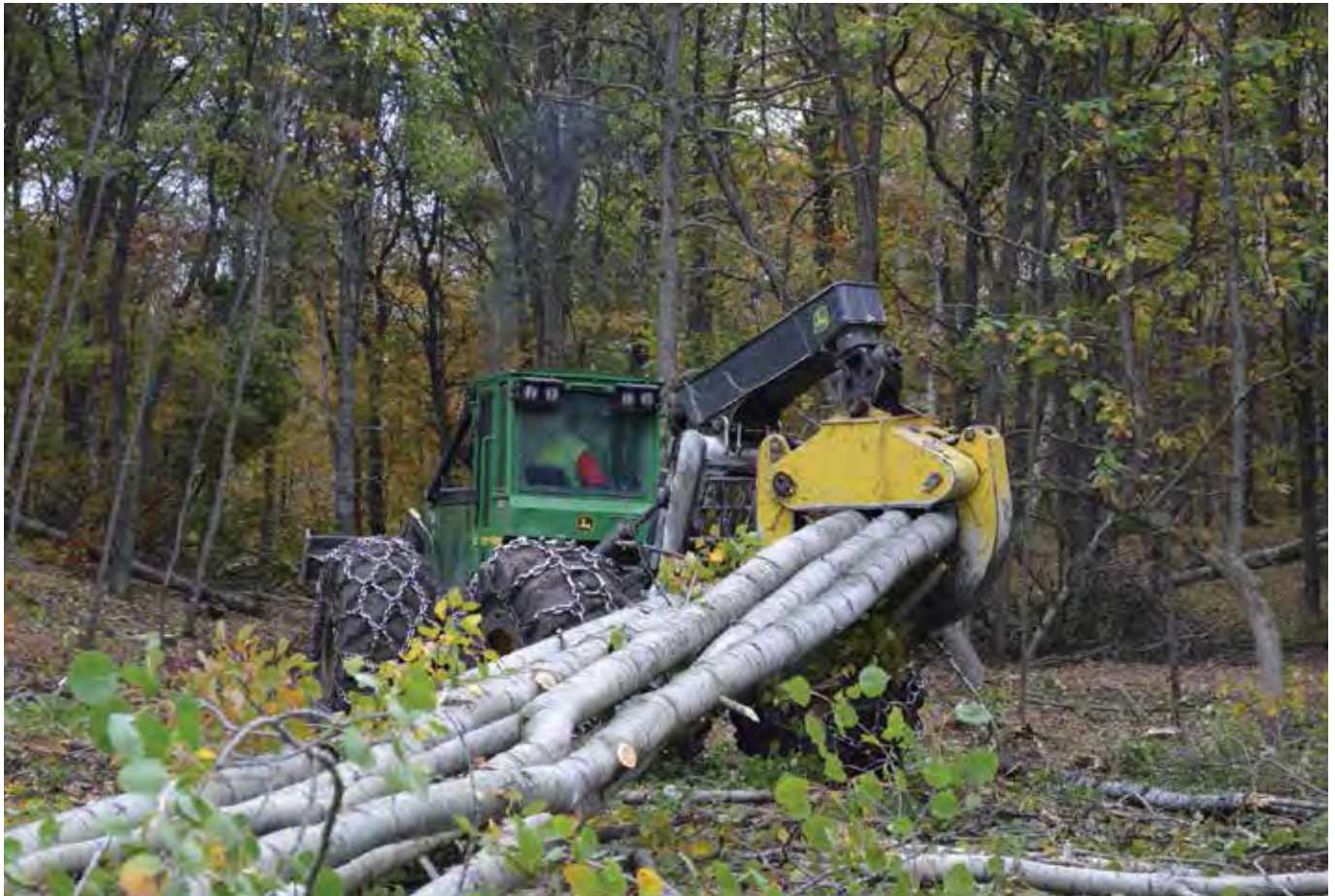
After delimiting the tree-length aspen, Tibbetts uses a John Deere 648H skidder to bring the wood to the landing for slashing and hauling.
