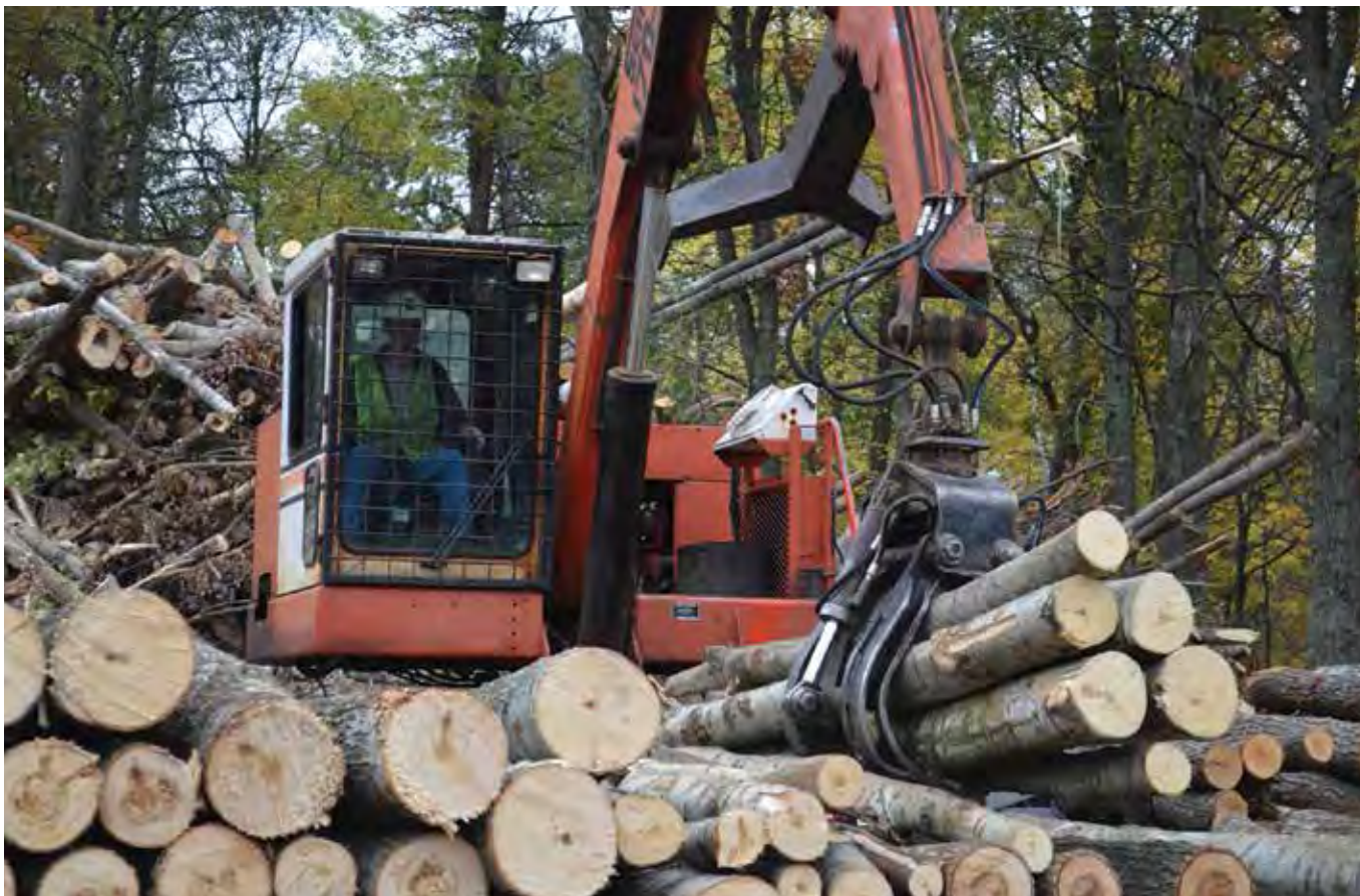
After slashing raw aspen into hundred-inch lengths, Bill Hettver piles the timber with a Serco 170-A slasher/loader so it can be easily loaded onto trucks for transport to market.
