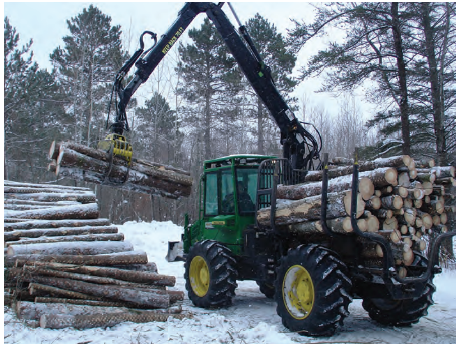
Eric Jemtrud off-loads harvested timber from the John Deere forwarder so it can be trucked to the mill.
