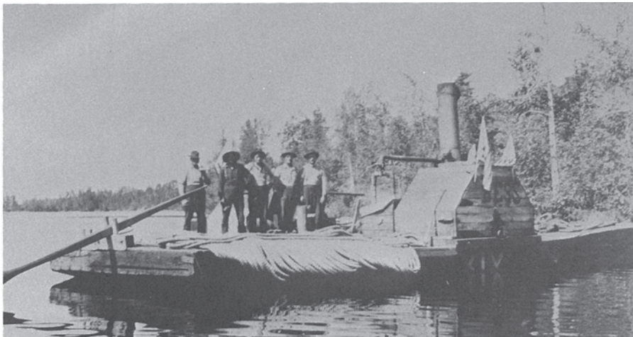
A steam "alligator" used by Virginia Rainy Lake Co. to tow logs to hoist.
