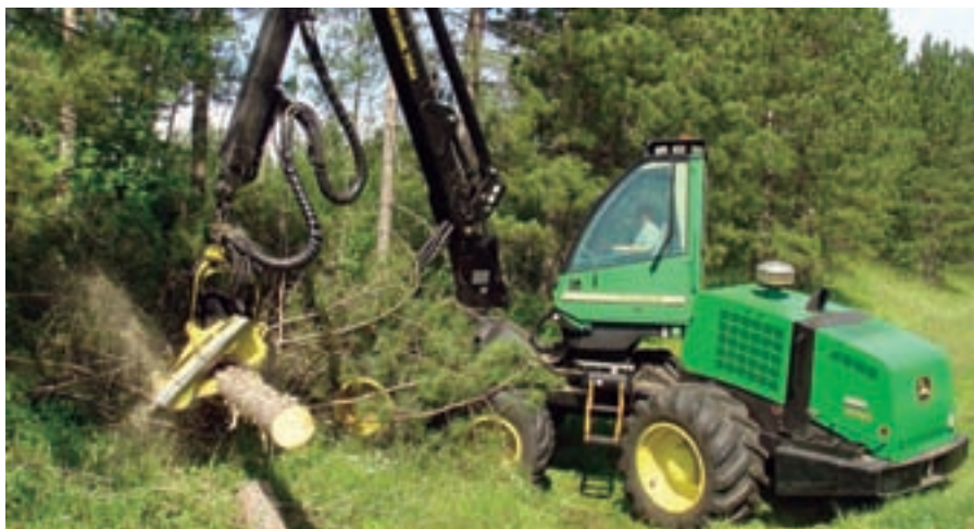
Moe Logging's John Deere 1270D harvester. Most of the time the harvester has tracks and chains, but for this job the Moes are operating with tires so they can move back and forth across the pavement.
