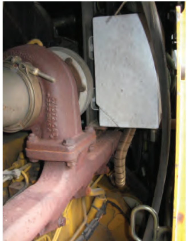
Example of discharging into the engine compartment – not recommended.
