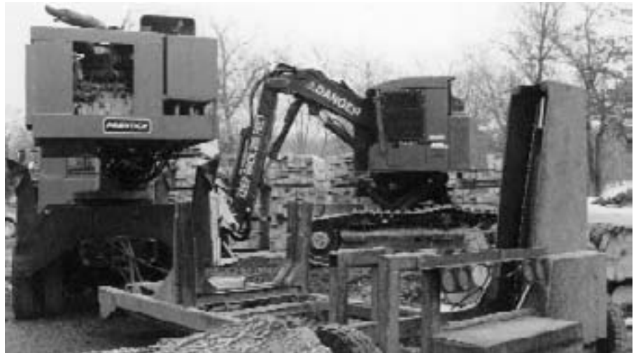
CRT slasher with 55-inch bar saw. Carriage is marked to cut 10-, 12- and 14-foot logs with the bang board horizontal.
