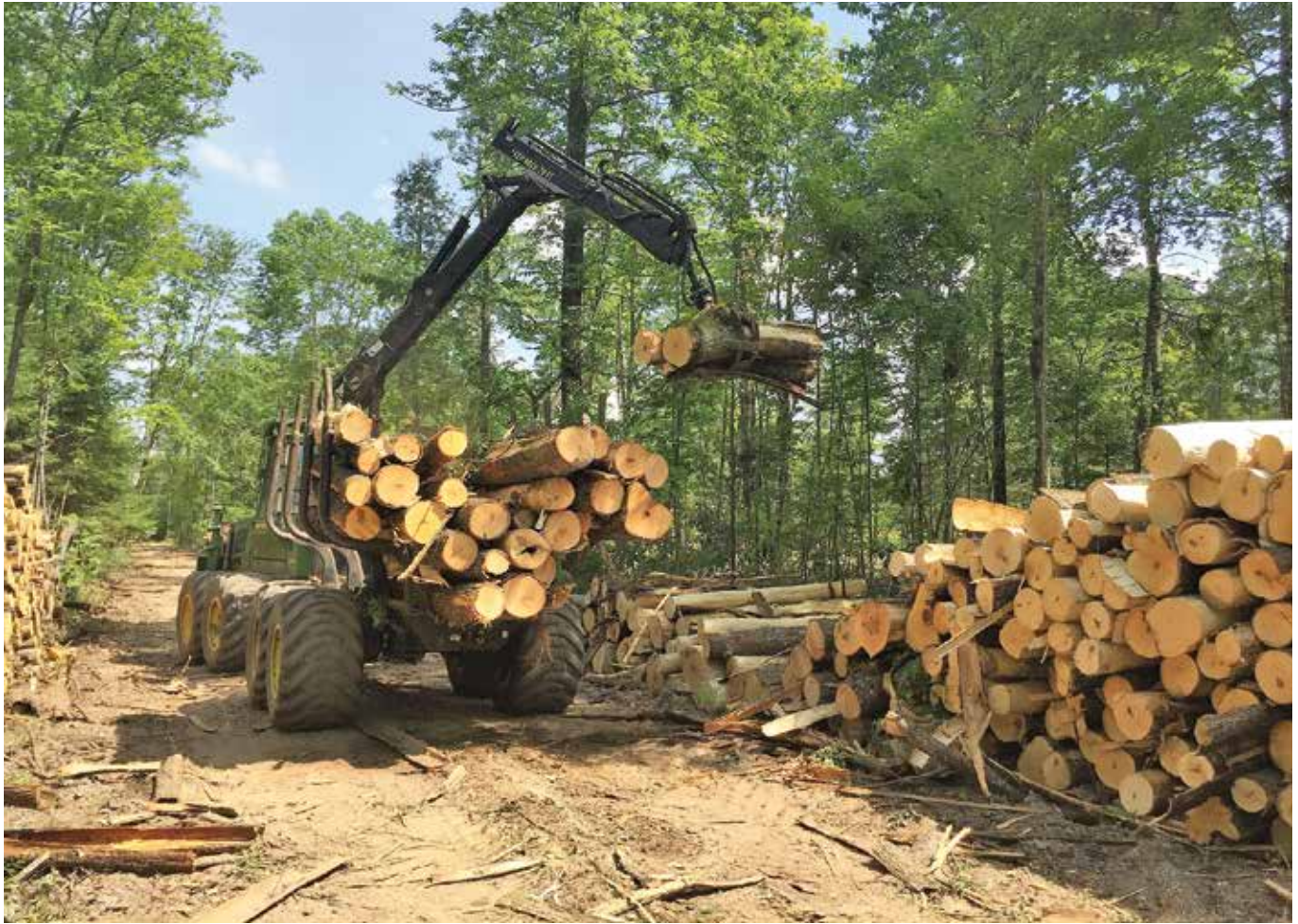
Richard Castile piles harvested aspen on the landing with a John Deere 1110 forwarder.
